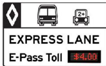
Figure 29: Dedicated dynamic message sign
