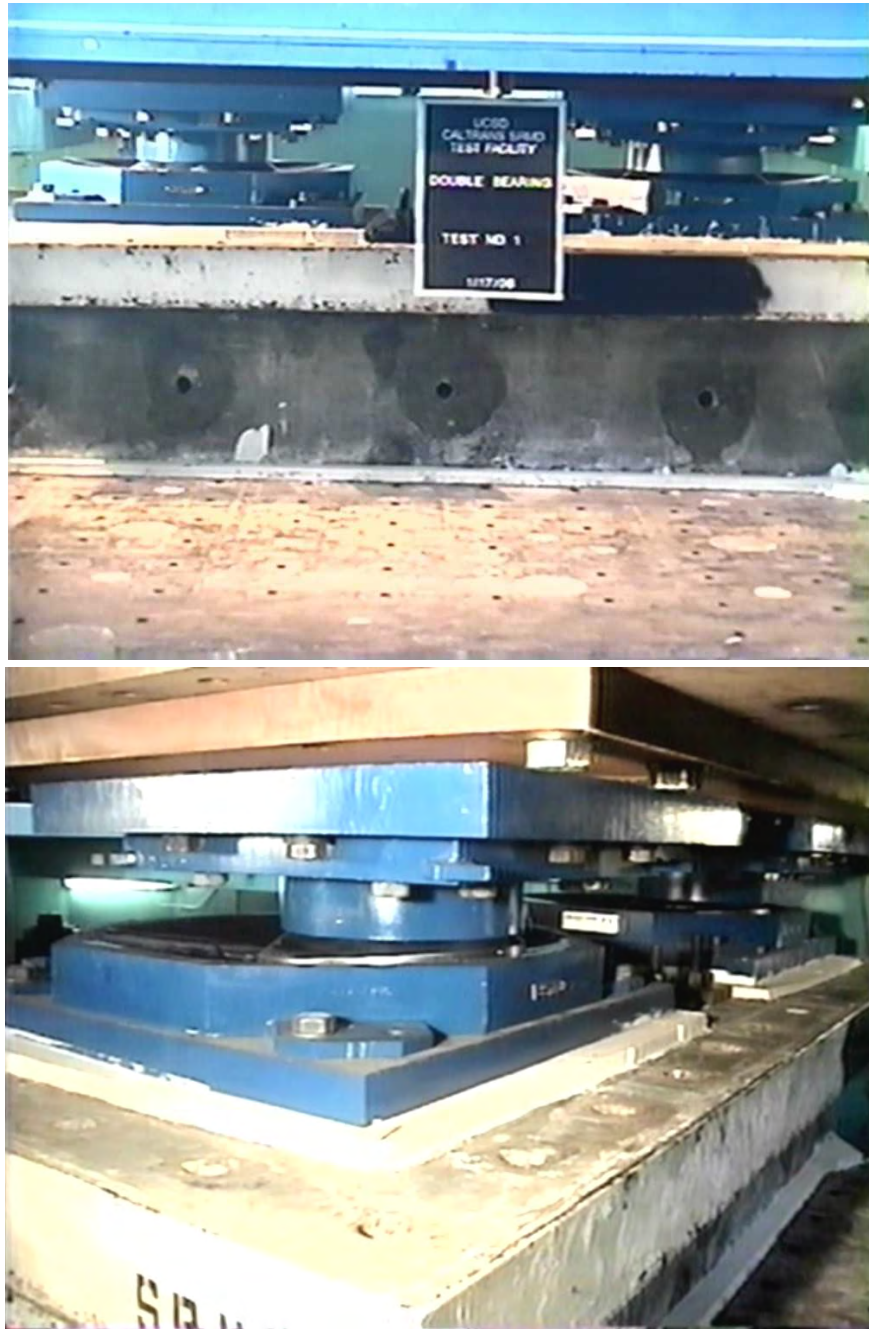
Figure 48 Overview of test setup at zero and maximum displacement.
