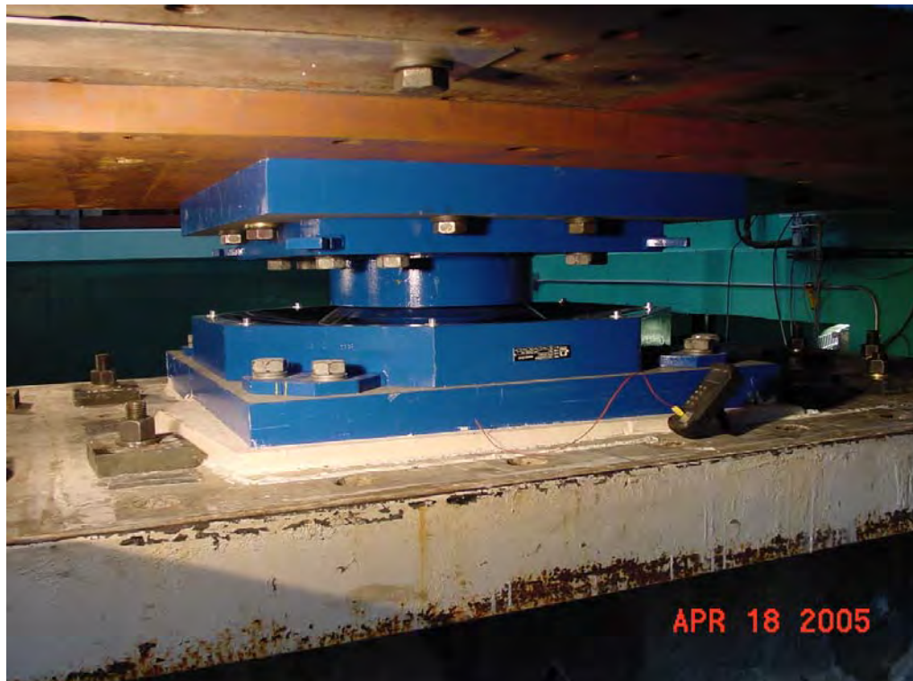
Figure 23 Typical sliding bearing installation
