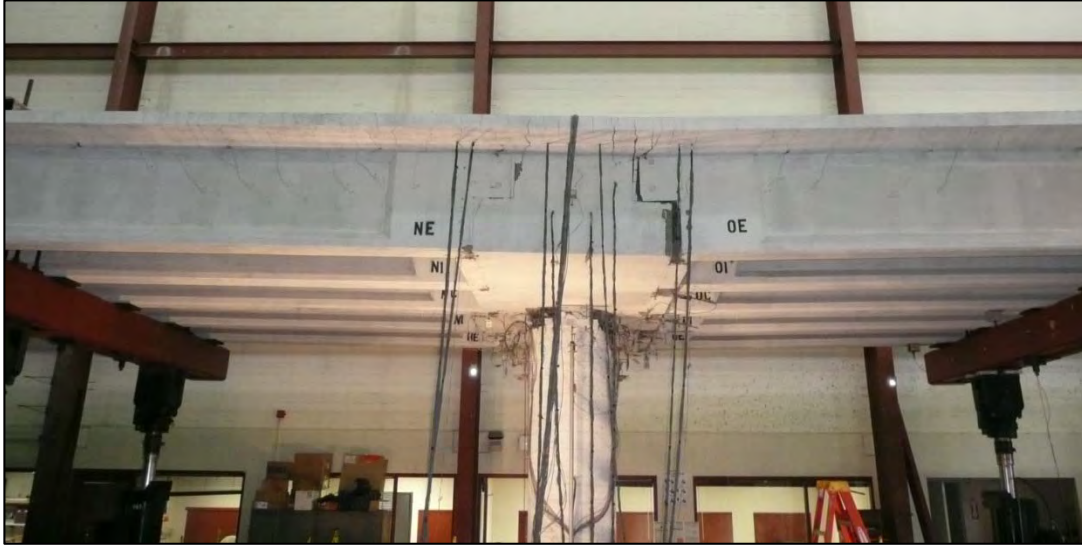
Figure 6.37: Overall Response of Test Unit at +3 in. of Vertical Displacement
