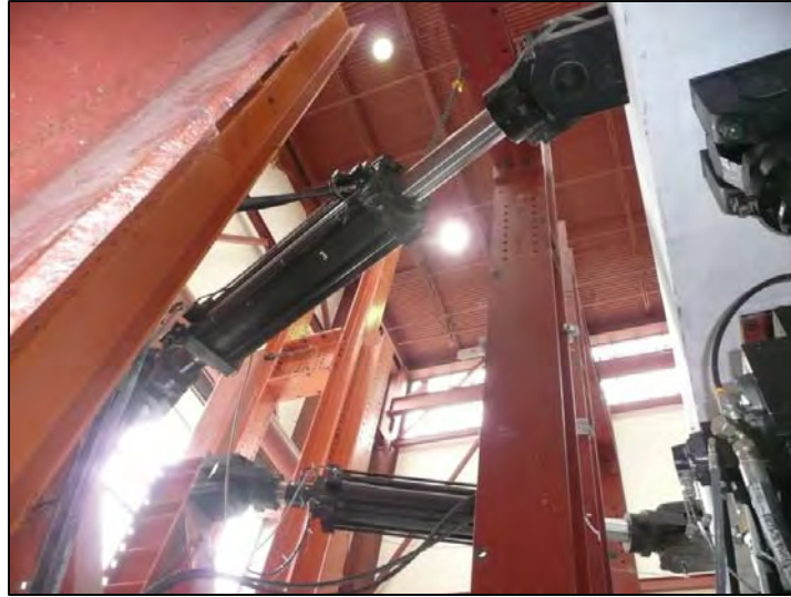
Figure 5.48: Horizontal Actuator Configuration used during Phase 1 Testing at Each End of the Test Unit
