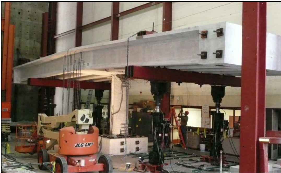
Figure 6.36: Displaced Test Unit at -6 in. of Displacement
