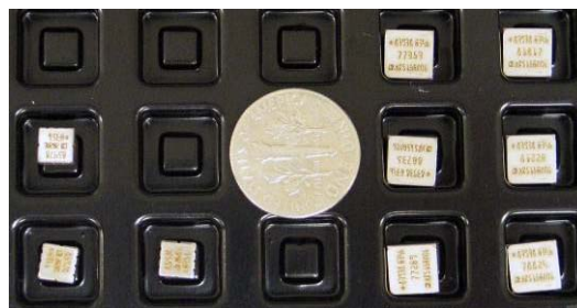
Figure 4: Analog Devices MEMS gyro and accelerometer chips
