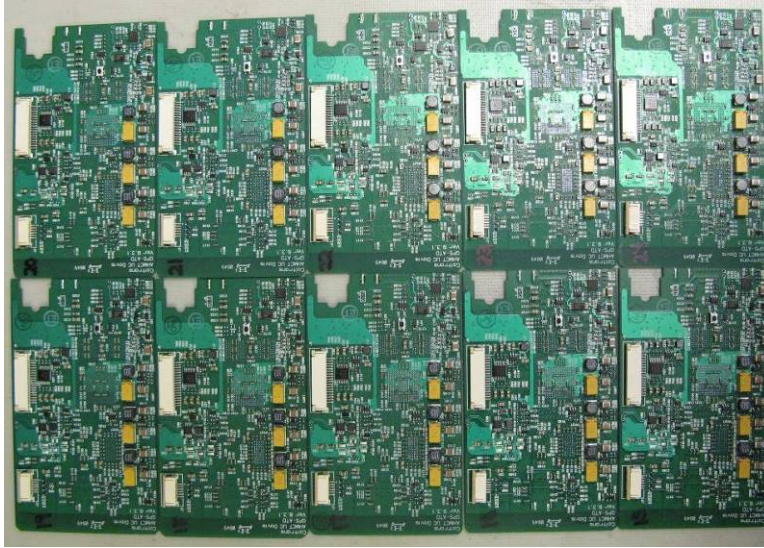
Figure 24: Fully-assembled GPS-ATD bottom-side circuit boards (qty 10 shown)
