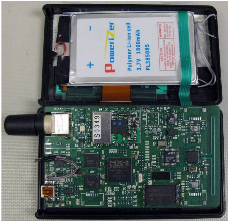
Figure 25: Fully-assembled GPS-ATD unit internals
