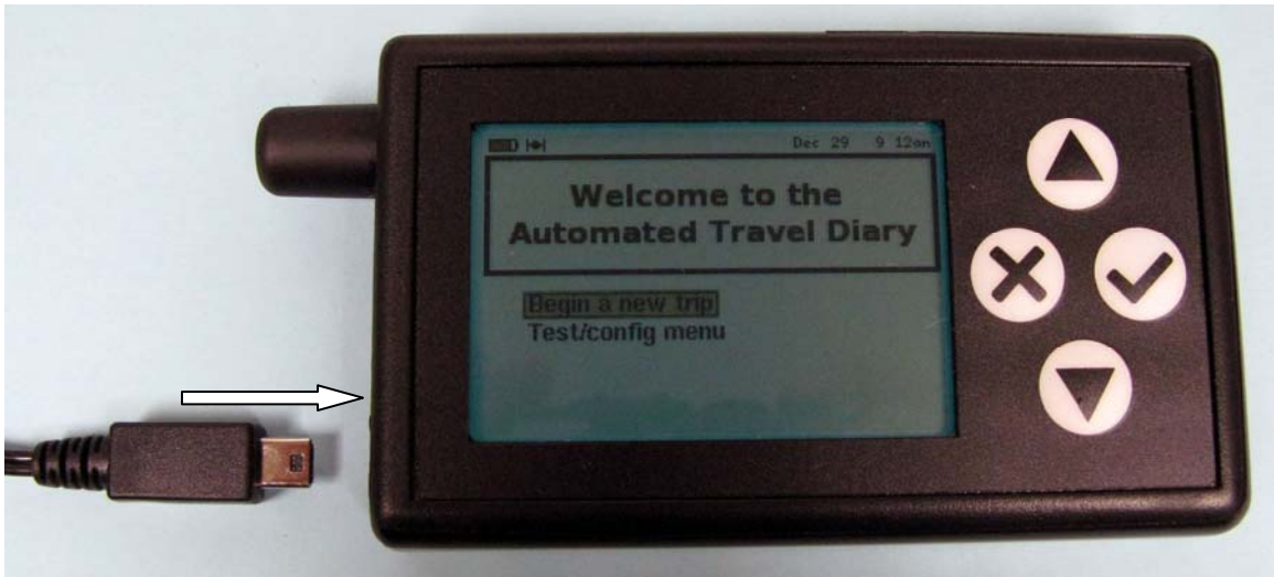
Figure 3: Charging the GPS-ATD
