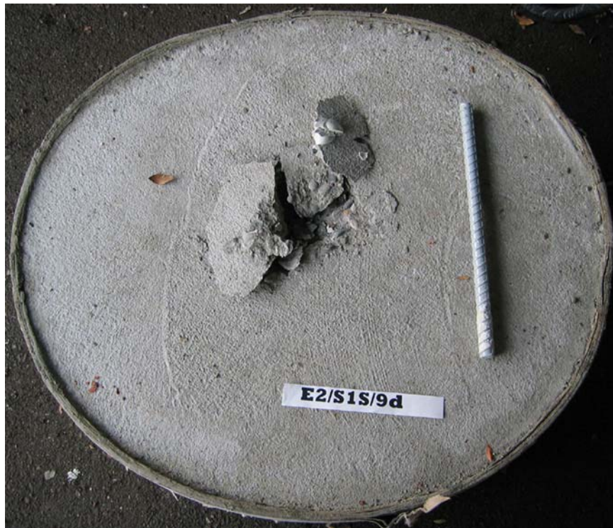
Figure A-4: Typical Adhesive/Rebar Interface Failure
