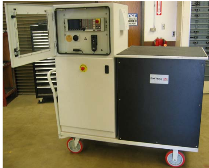
Figure 5-2: Cart with Controller and Hydraulic Pump
