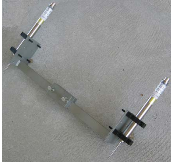
Figure 5-5: LVDT Bracket for Creep Testing
