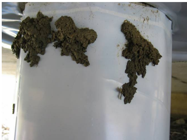
Figure 7. Mud sliding down surface of PTFE surface modification on column.
