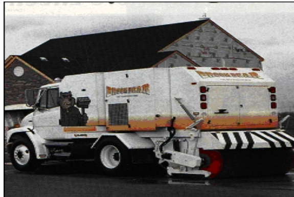
Figure 9-27 Sweeping with a Suction Broom
