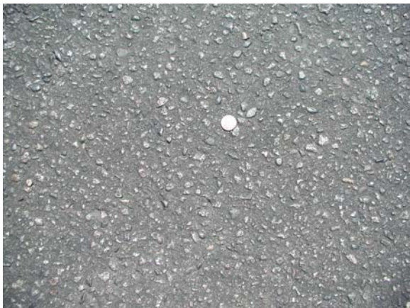
5 year old DGAC surface. Aggregate is exposed but surface is tight .Emulsion will not penetrate. Not suitable for fog seal or rejuvenator seal.
