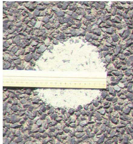
b) Sand Patch Test
