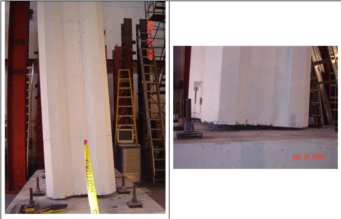
Figure 9.26 Column displacement and pin rotation close-up
