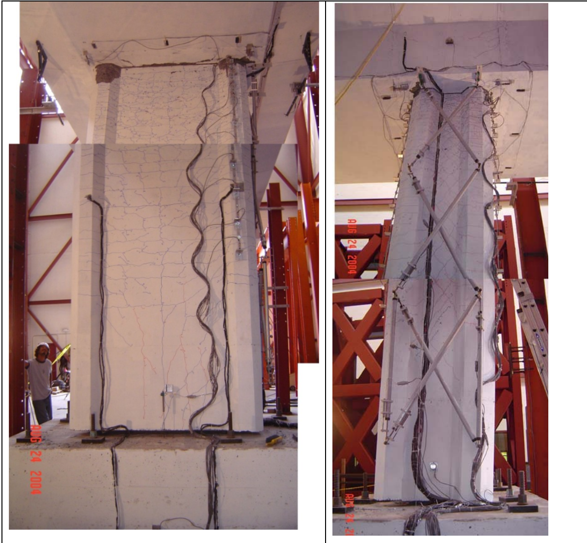
Figure 6.8 Marked crack pattern on north and west faces of column at \mu=8
