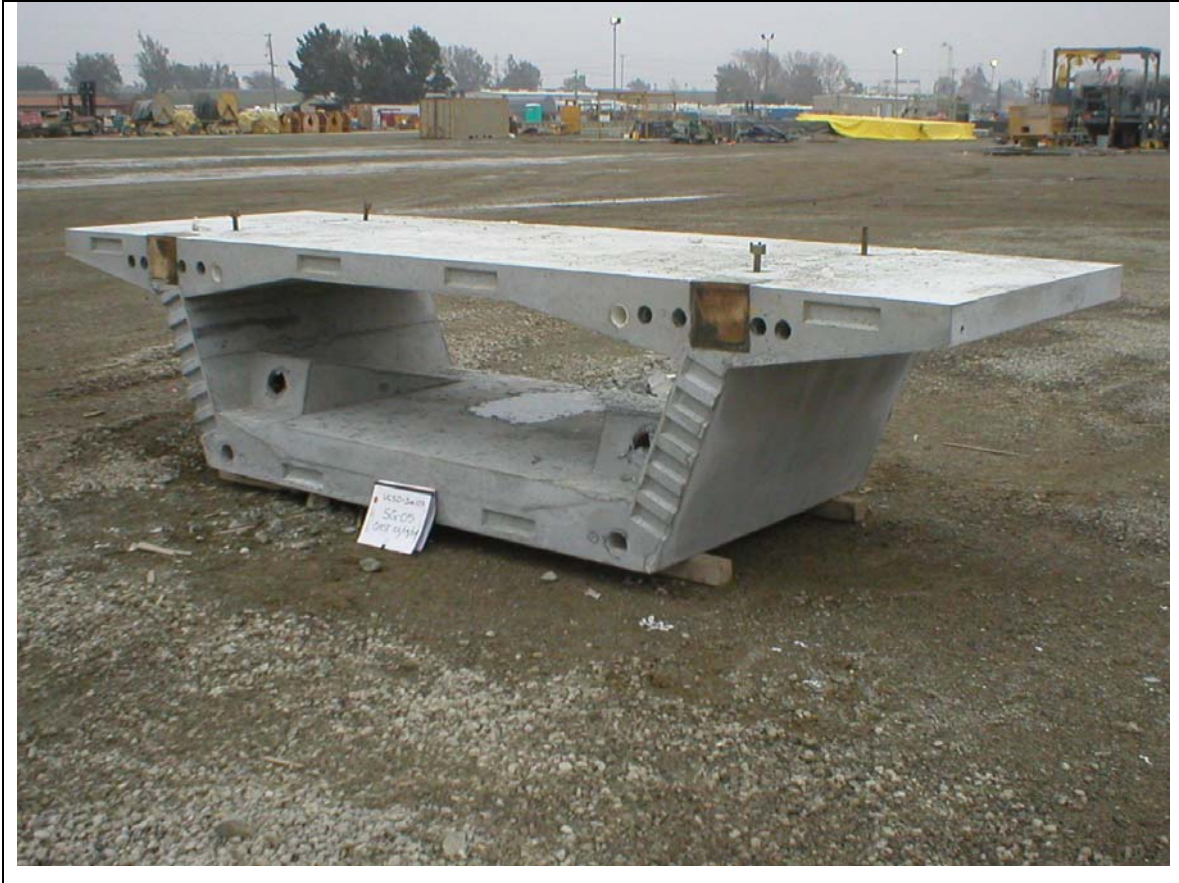
Figure 9.11 First completed segment (later scrapped because the bottom blisters are backwards)
