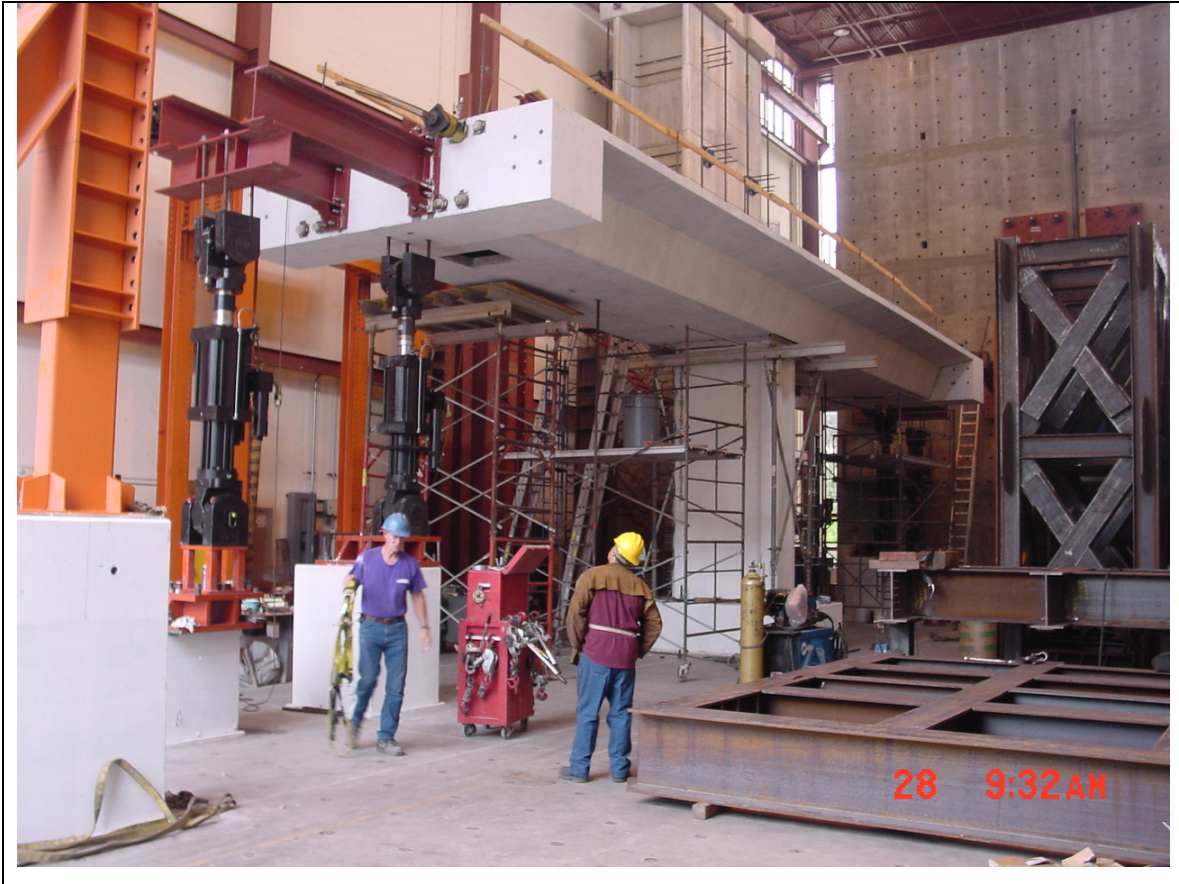
Figure 9.23 Test during placement of actuators
