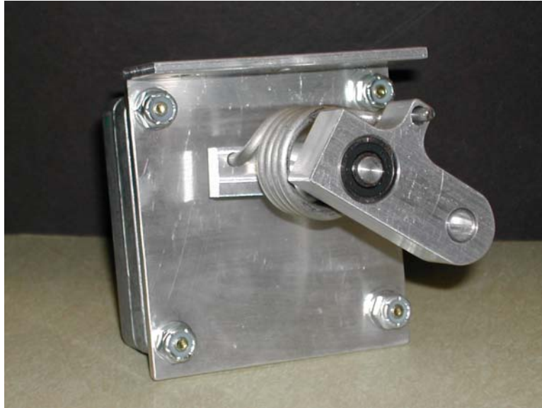
Figure 9.10: Brake with bent spring
