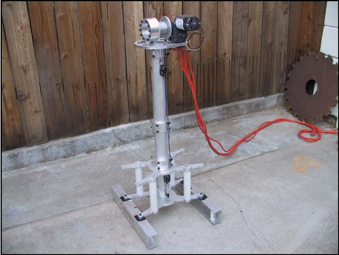
Figure 3.5, Deployable Trolley-ABDS Lifting Mechanism
