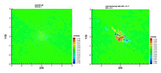
Figure 4. Cross sectional contours of normalized mean streamwise vorticity at x/D = 0.1.
