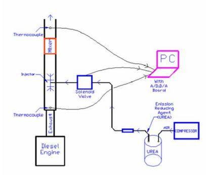
Figure 3. Air-Assisted Injection System.
