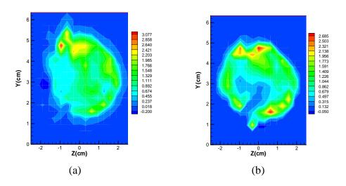
Figure 13. Contours of (a) primary turbulent shear stress, uv\*100/Uo^2, (b) secondary turbulent shear stress, uw\*100/Uo^2. m=0.15, x/D=0.1.
