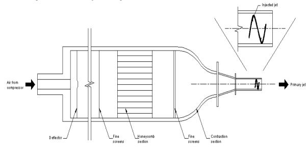
Figure 2. Experimental Set-up.
