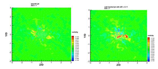
Figure 5. Cross sectional contours of normalized mean streamwise vorticity at x/D = 1.
