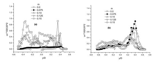
Figure 9. Variation of turbulent shear stress along the mid-section for different injection ratios. (a) x/D = 0.1, (b) x/D = 1.
