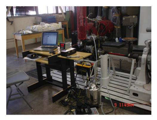
Figure 17. Diesel Engine and the SCR system.
