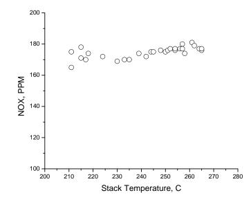
Figure 18. Exhaust NOx without Urea Injection.
