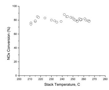
Figure 19. NOx Conversion with Urea Injection.
