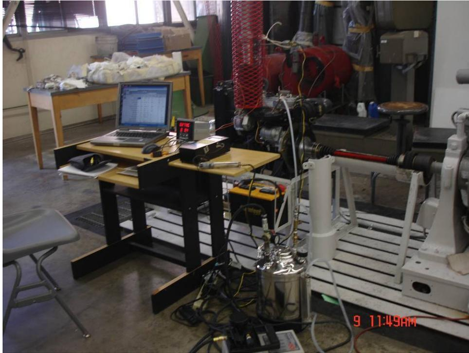
Figure 17. Diesel Engine and the SCR system.
