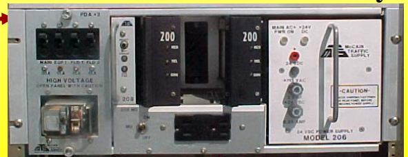
Power Distribution Assembly
