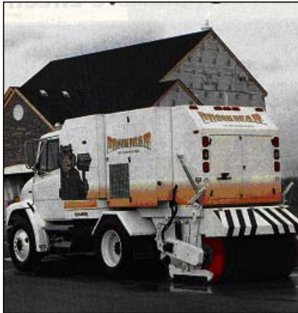
Figure 27: Sweeping with a Suction Broom
