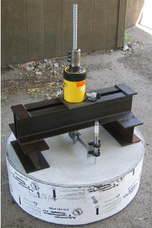
Figure 5-4: Creep Loading Setup
