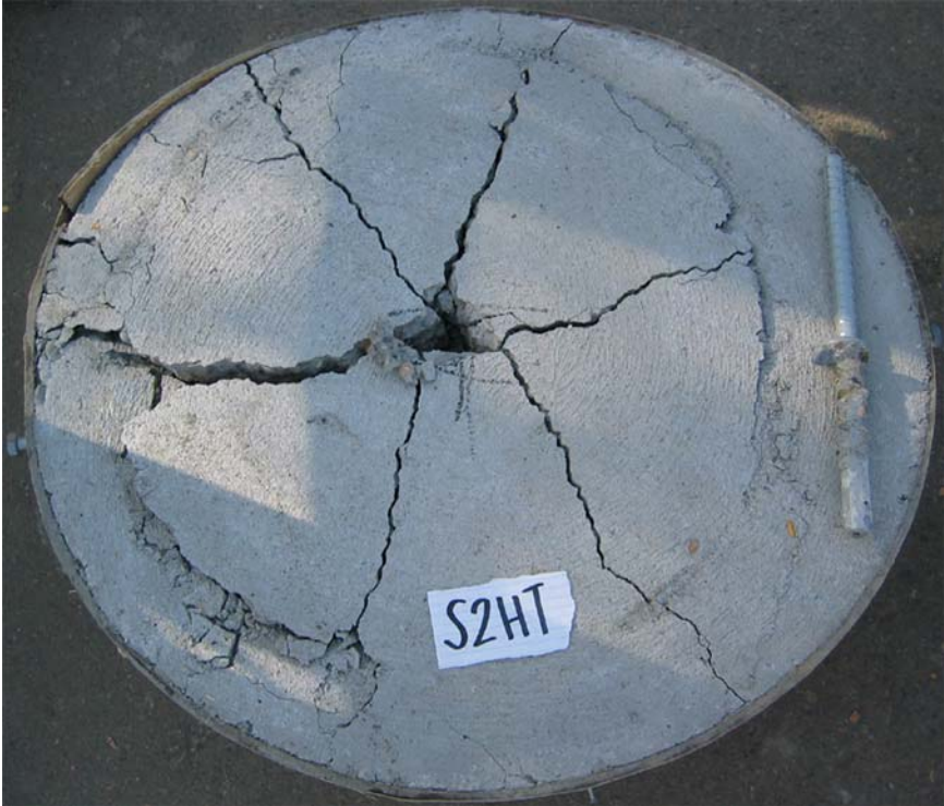
Figure A-1: Typical Concrete–Concrete/Adhesive Interface Failure
