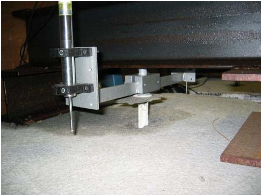
Figure A-6: Red Head C6 Creep Failure
