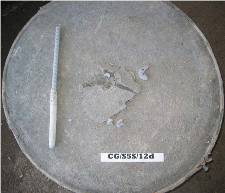
Figure A-2: Typical Concrete/Adhesive Interface Failure
