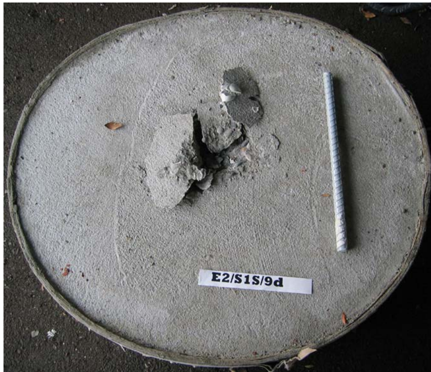
Figure A-4: Typical Adhesive/Rebar Interface Failure
