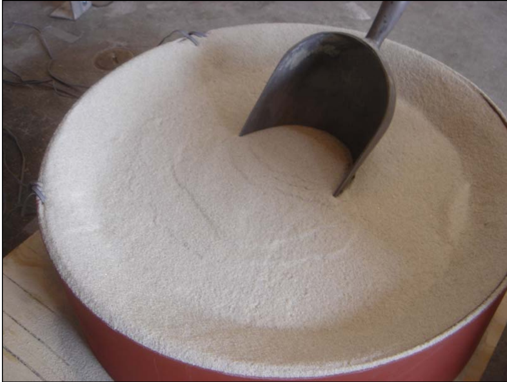
Figure 4.24: The filler material has developed a significant soil fabric.
