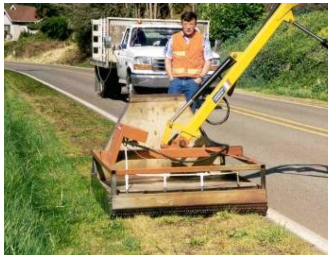
Figure 2.7 Infrared vegetation control unit
