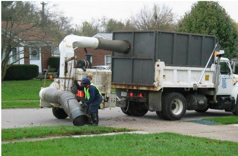
Figure 3.1 Workers guiding vacuum tip to remove leaf piles.
