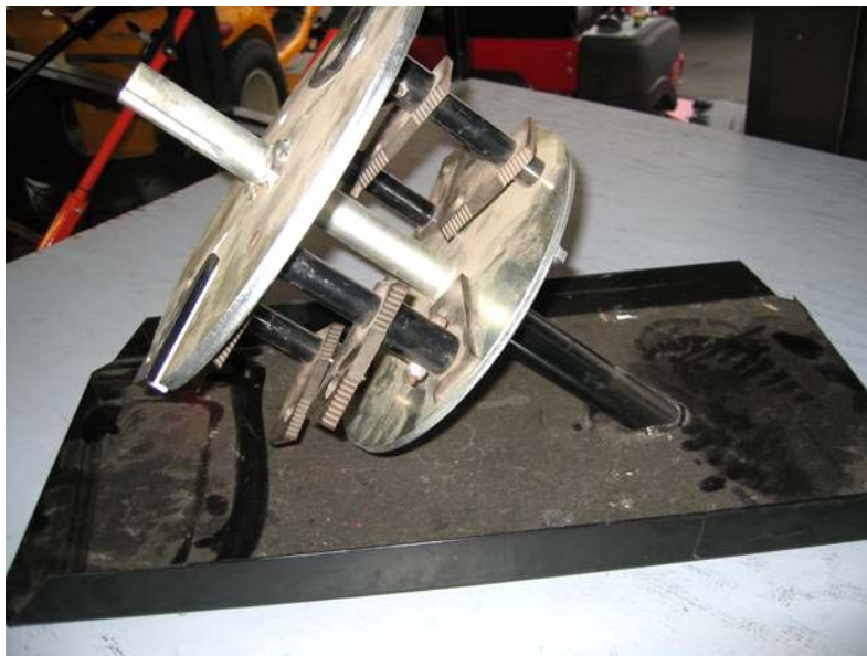
Figure 8.1 Cutting wheel from a commercial Chipper/Shredder
