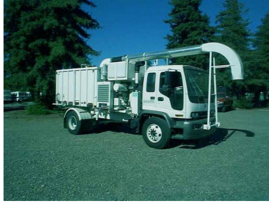
Figure 3.2 Fixed boom vacuum vehicle.
