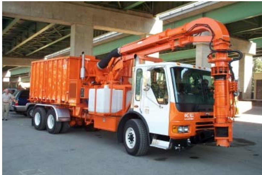
Figure 1.1 ARDVAC Attached to Boom Vacuum Truck
