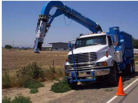
Figure 3.3 Industrial vacuum vehicle with articulated boom.
