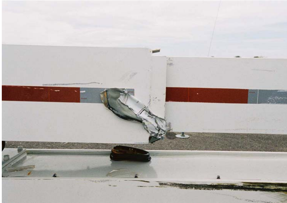
Figure 2-18 Barrier After Test 641
