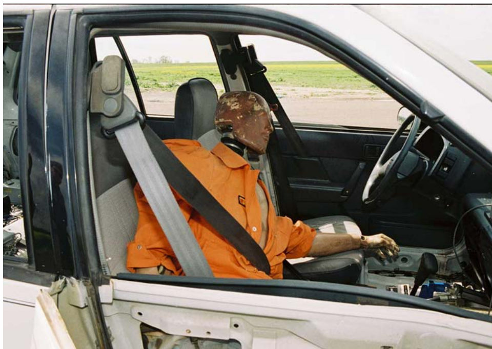
Figure 2-19 Final Resting Place of Test Dummy
