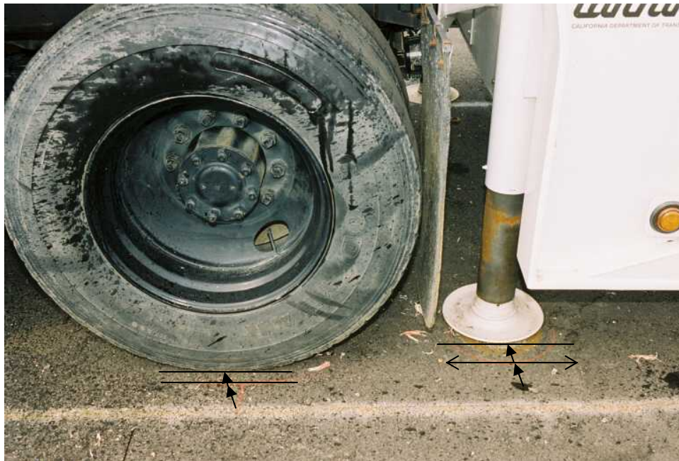
Figure 2-32 Trailer Tire and Brace Displacement in Test 642
