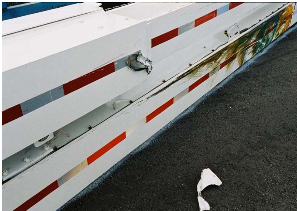
Figure 2-17 Barrier After Test 641
