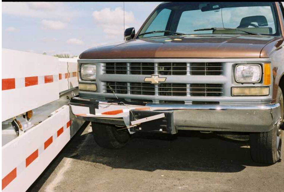
Figure 2-23 Close-up of Impact Area Prior to Test 642
