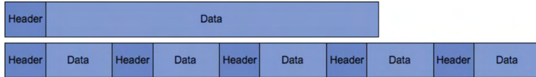
Figure 26: Illustration of transmission of one 250B packet and five 50B packets
