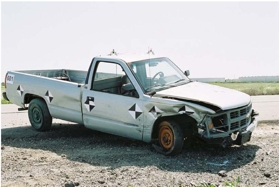
Figure 2-10 – Front Right Corner of Test Vehicle Post-Impact
