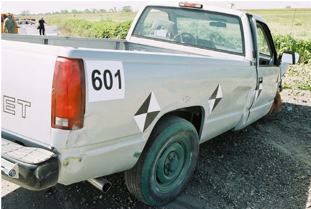
Figure 2-11 – Rear Right Side of Test Vehicle Post-Impact
