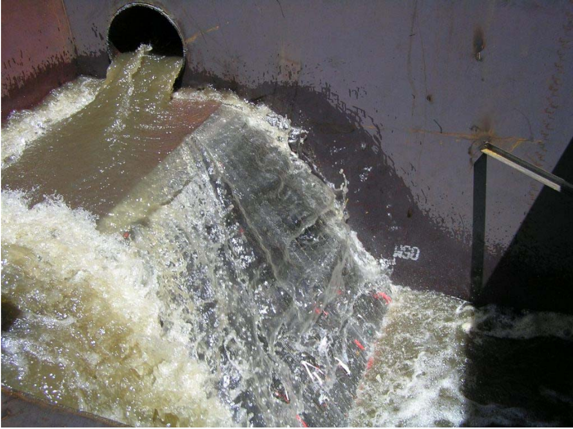
Fig. 6.16: Flow over screen at Q=3.5 cfs
