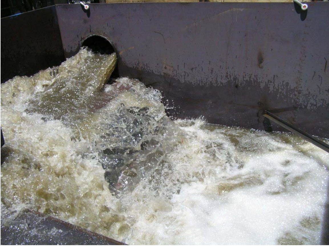
Fig. 6.30: Conditions in gross solids storage device for Q=9.0 cfs.
