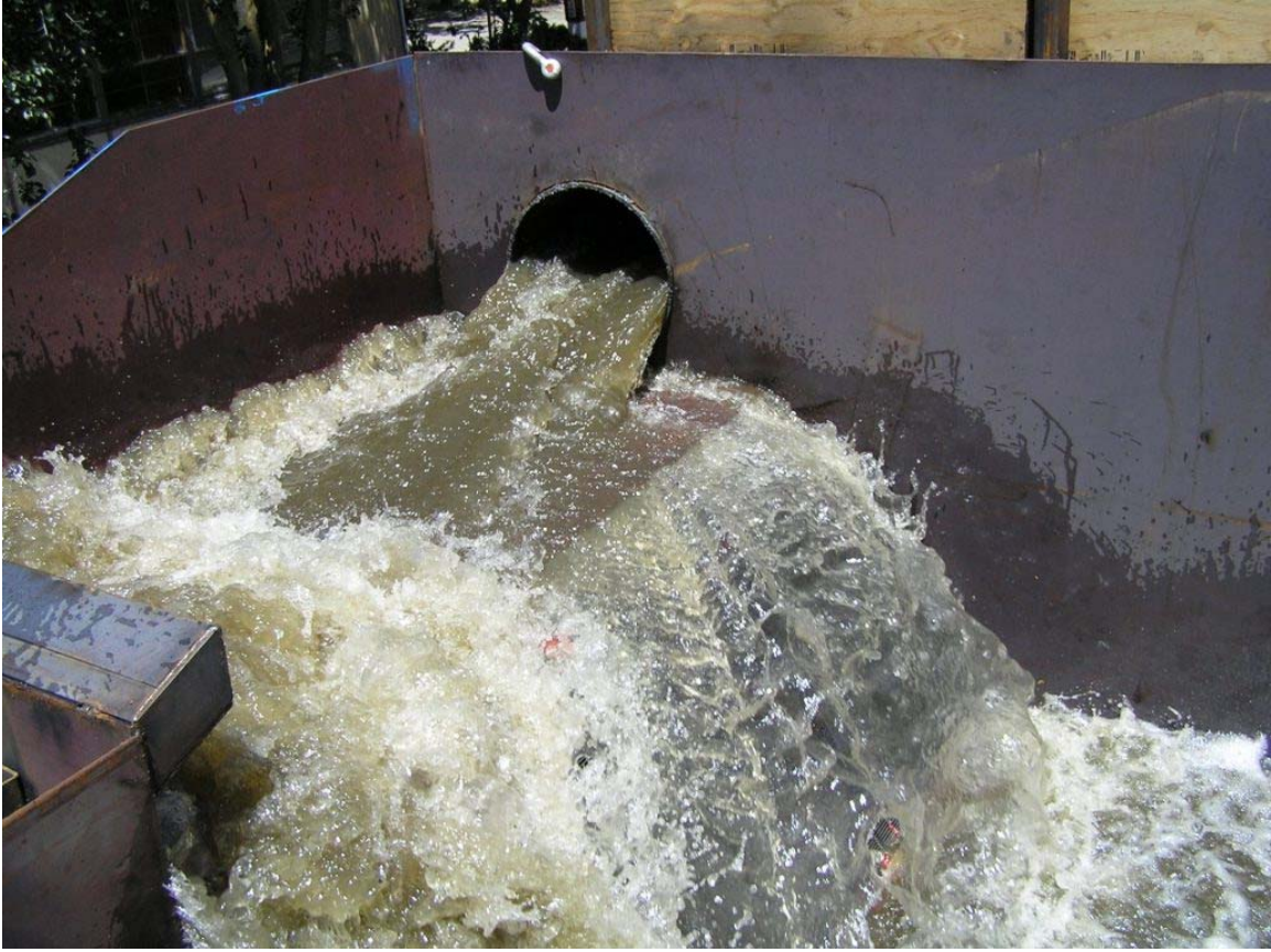
Fig. 6.23: Flow over shelf showing significant loss of screen conveyance efficiency.
