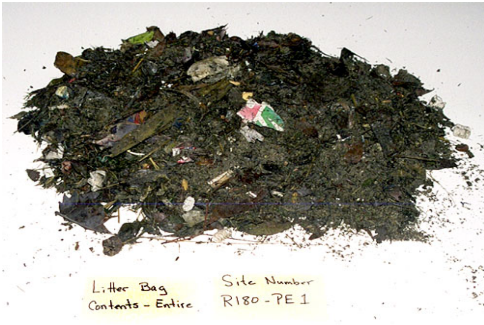
Fig 3.1: Gross solids including vegetation and sediment
