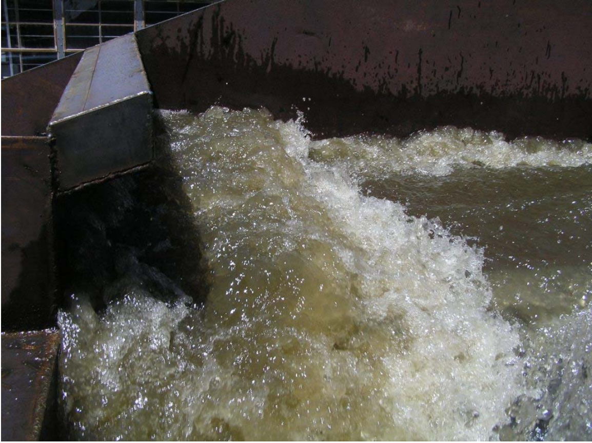
Fig. 6.19: View of water accumulation towards end of inflow shelf for Q=4.35 cfs.
