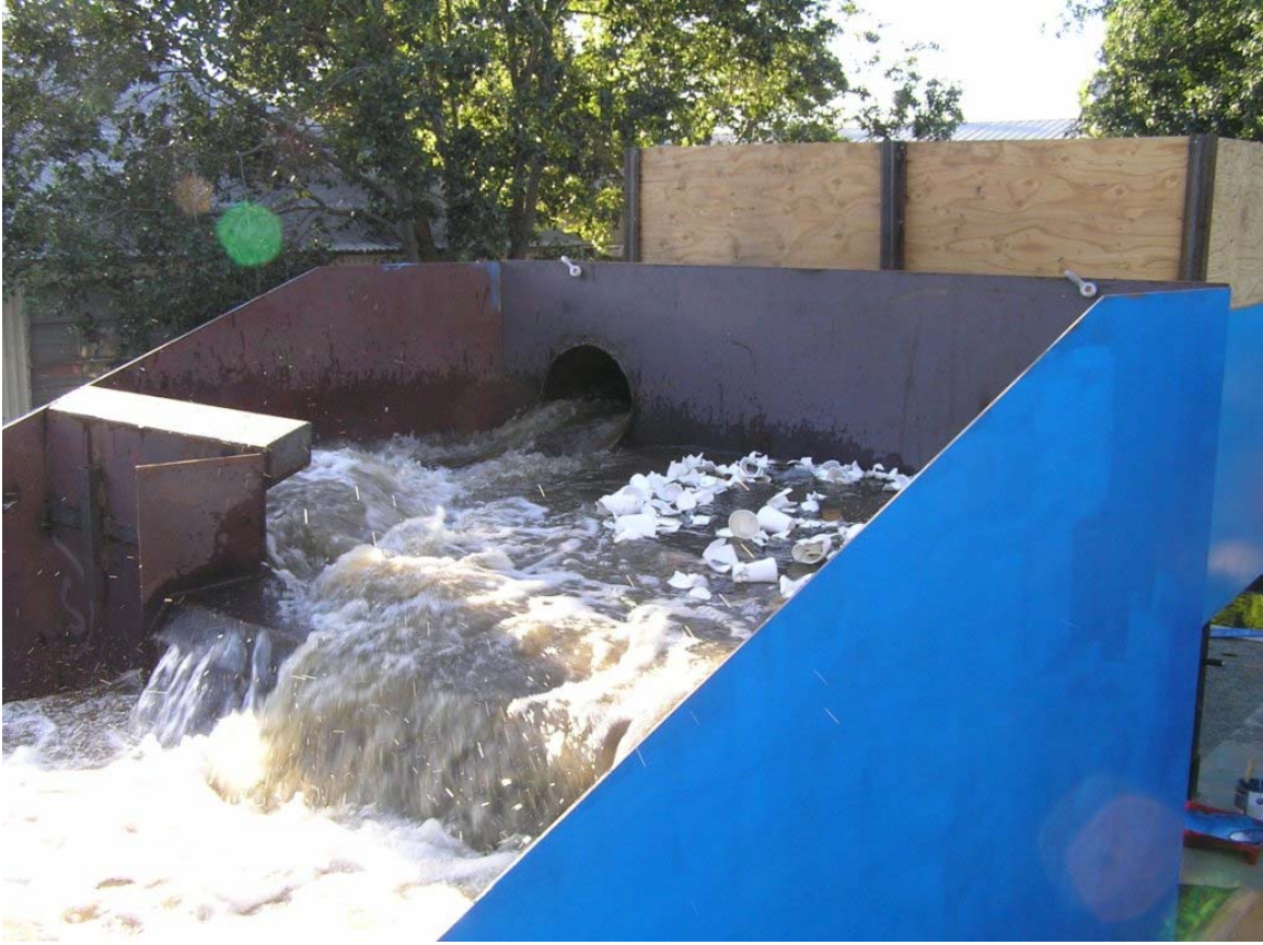
Fig. 6.46: Overflow for Q=5.5 cfs and 50% loading.
