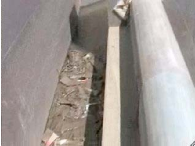
Fig. 5.12: Inflow trough storage after completion of test with Q=5.5 cfs and 50% loading.
