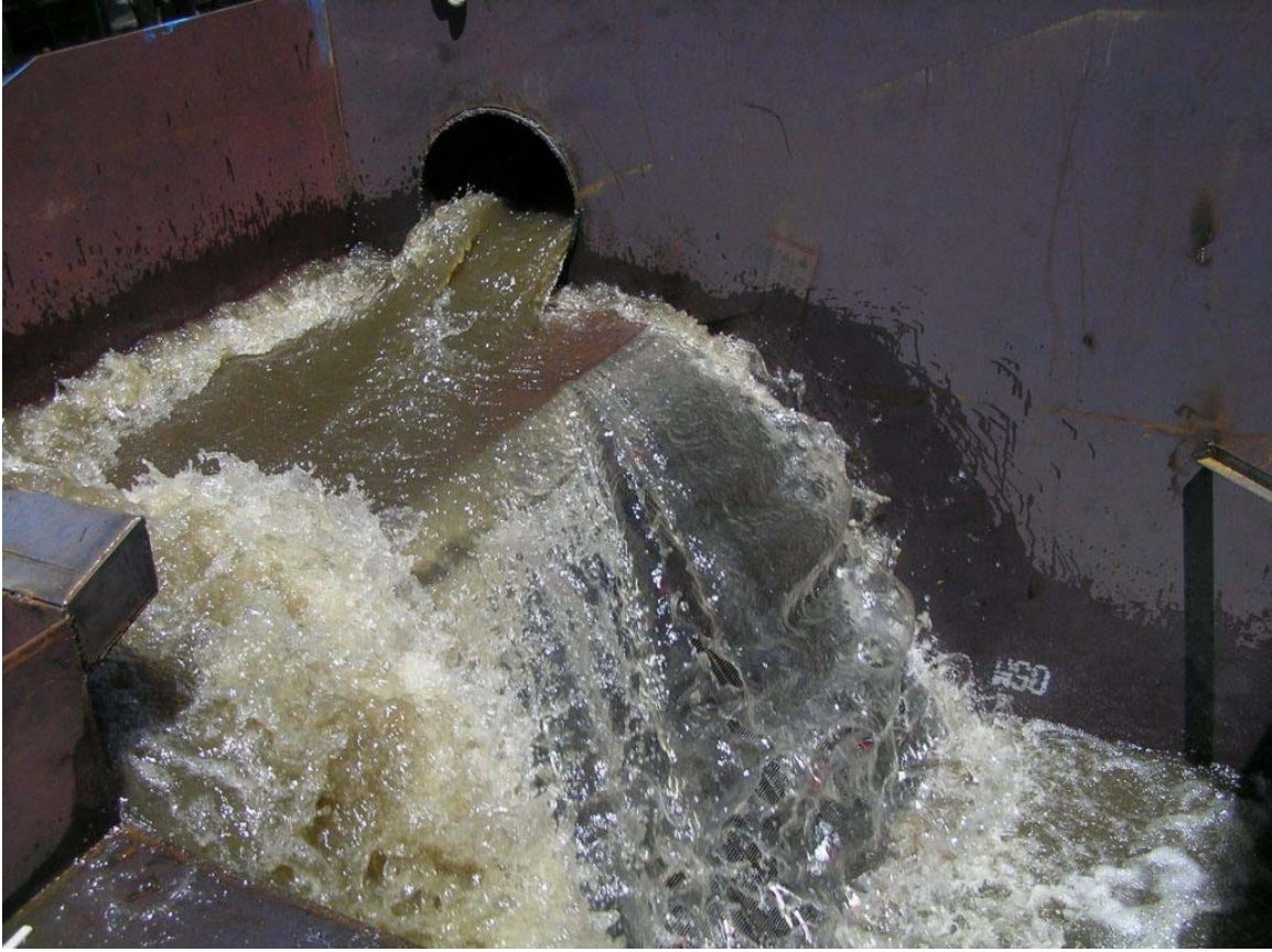
Fig. 6.18: Flow over screens for Q=4.35 cfs.
