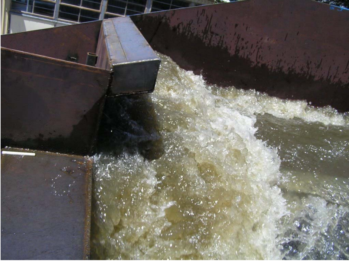
Fig. 6.21: Water surface elevation at splash shelf for Q=5.0 cfs.
