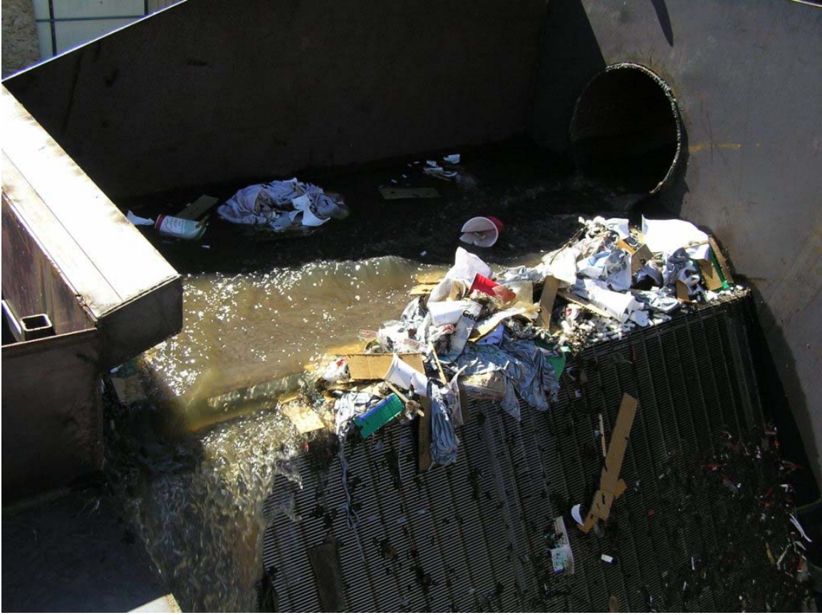
Fig. 6.37: Build-up of gross solids over portions of the screens ( Q=1.1 cfs, 50% loading).
