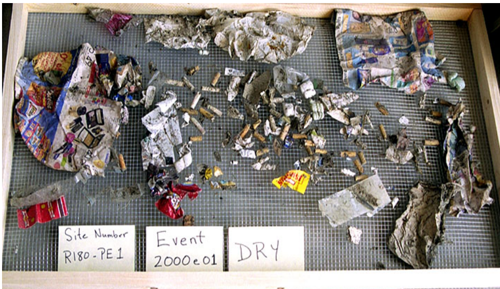
Fig. 3.2: Dry gross solids collected from Caltrans outfalls.
