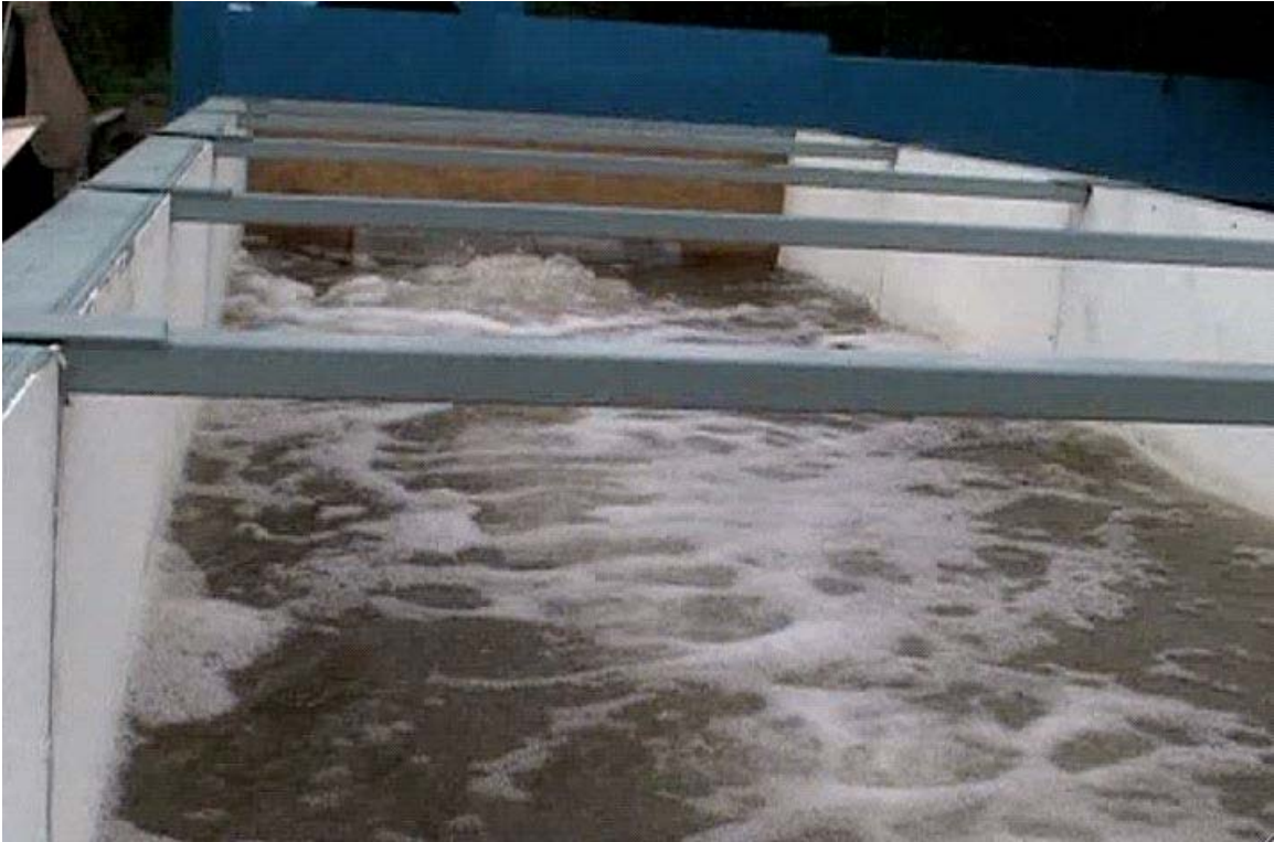
Fig. 4.57: Overflow for Q=29 cfs and 90% loading.
