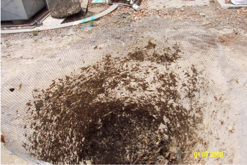
Fig. 2.13: 0.25" square wire mesh used for litter capture downstream of GSRD.
