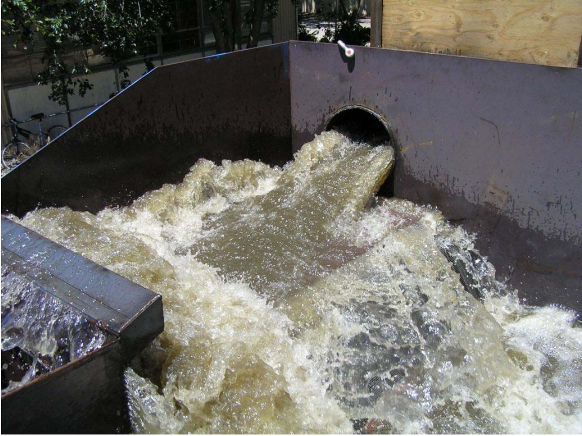
Fig. 6.29: Inlet conditions for Q=9.0 cfs.
