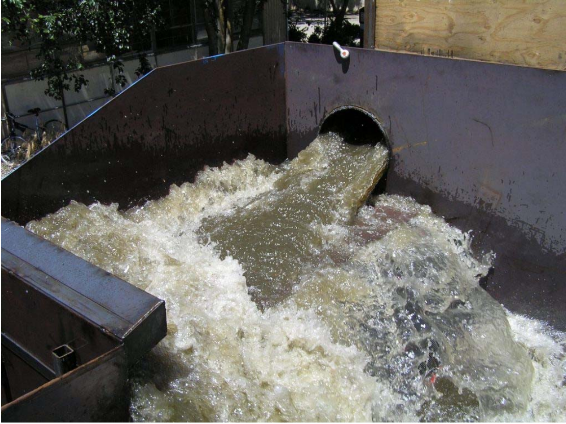
Fig. 6.28: Inflow conditions for Q=8.24 cfs.
