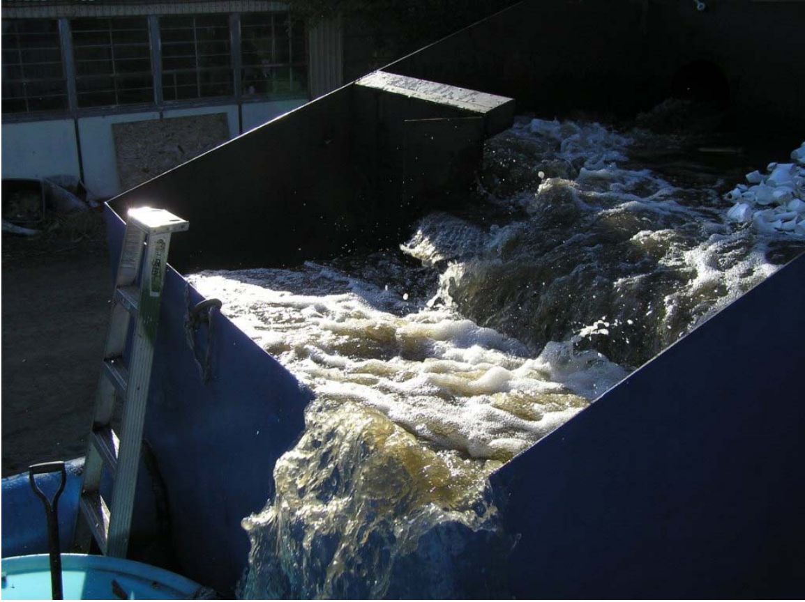
Fig. 6.47: Overflow for Q=5.5 cfs and 50% loading.
