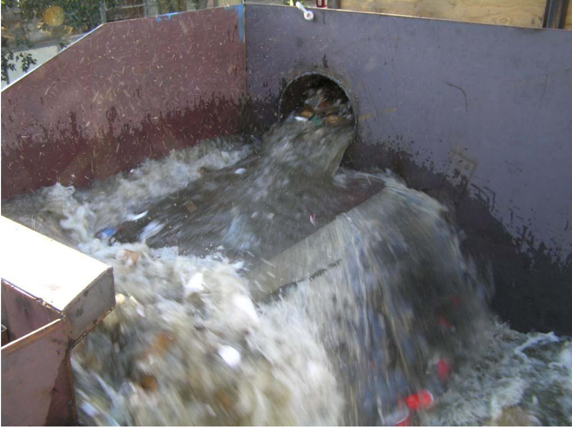
Fig. 6.43: Inflow patterns with Q=5.5 cfs and 10% loading.
