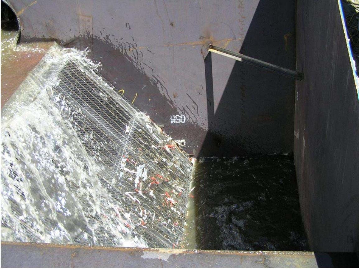
Fig. 6.12: Water distribution over screen for Q=1.85 cfs.
