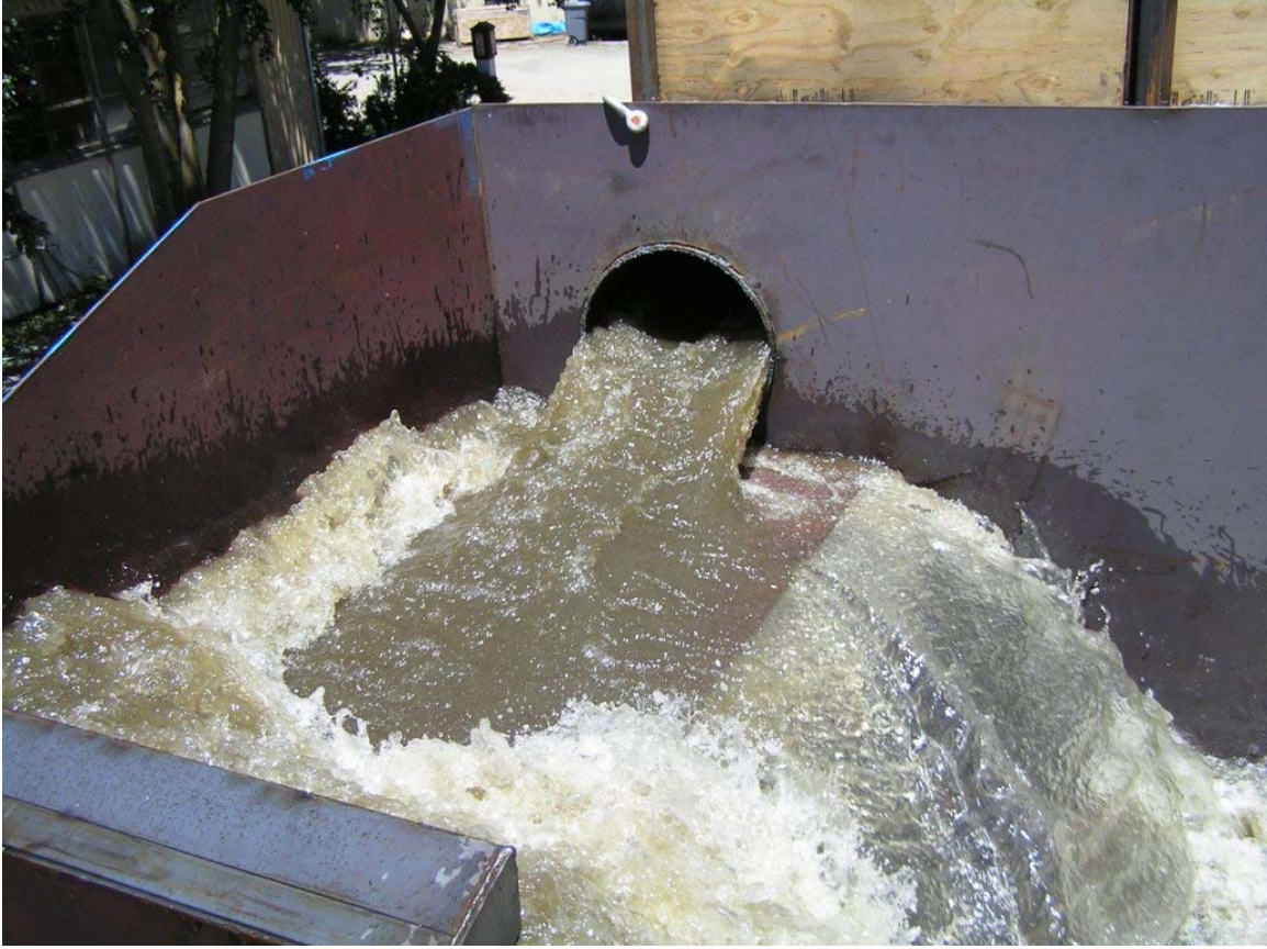
Fig. 6.25: Inflow conditions for Q=7.06 cfs.
