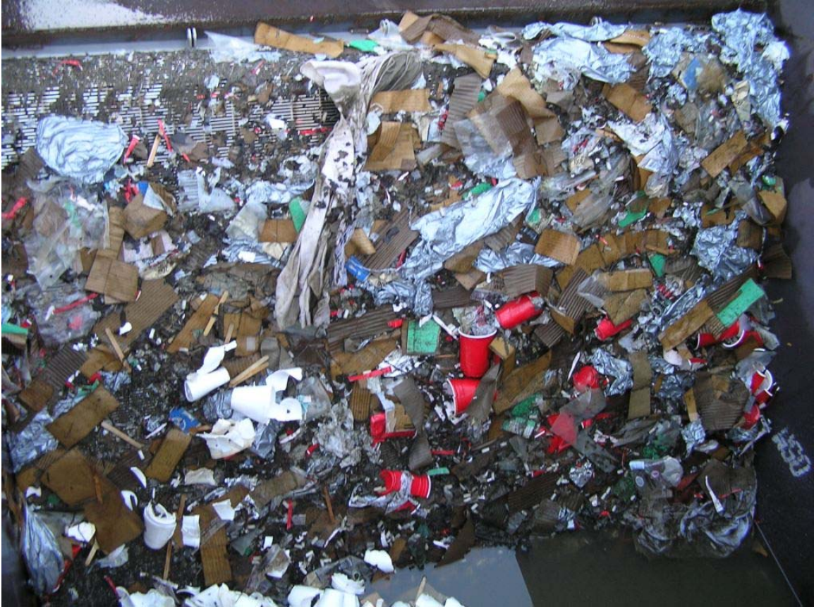
Fig. 6.51: Aftermath of Q=5.5 cfs and 50% loading.
