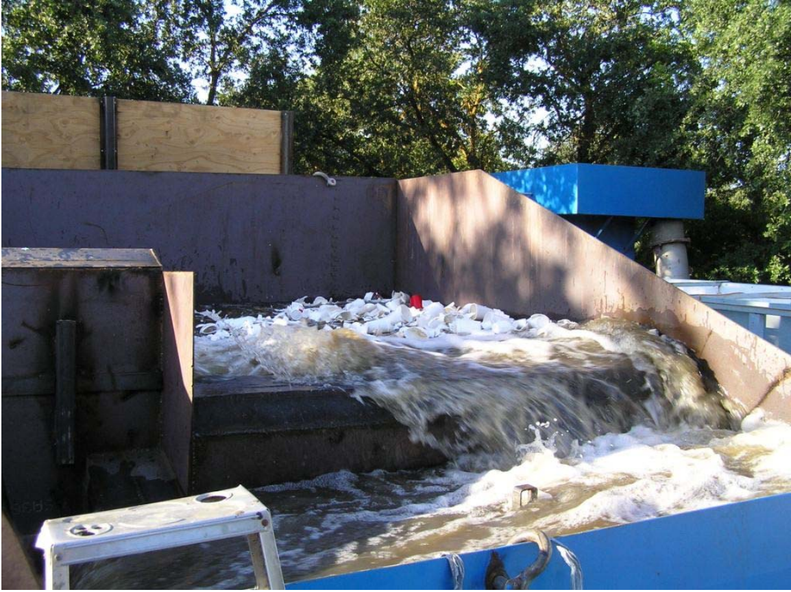
Fig. 6.45: Overflow for Q=5.5 cfs and 50% loading.
