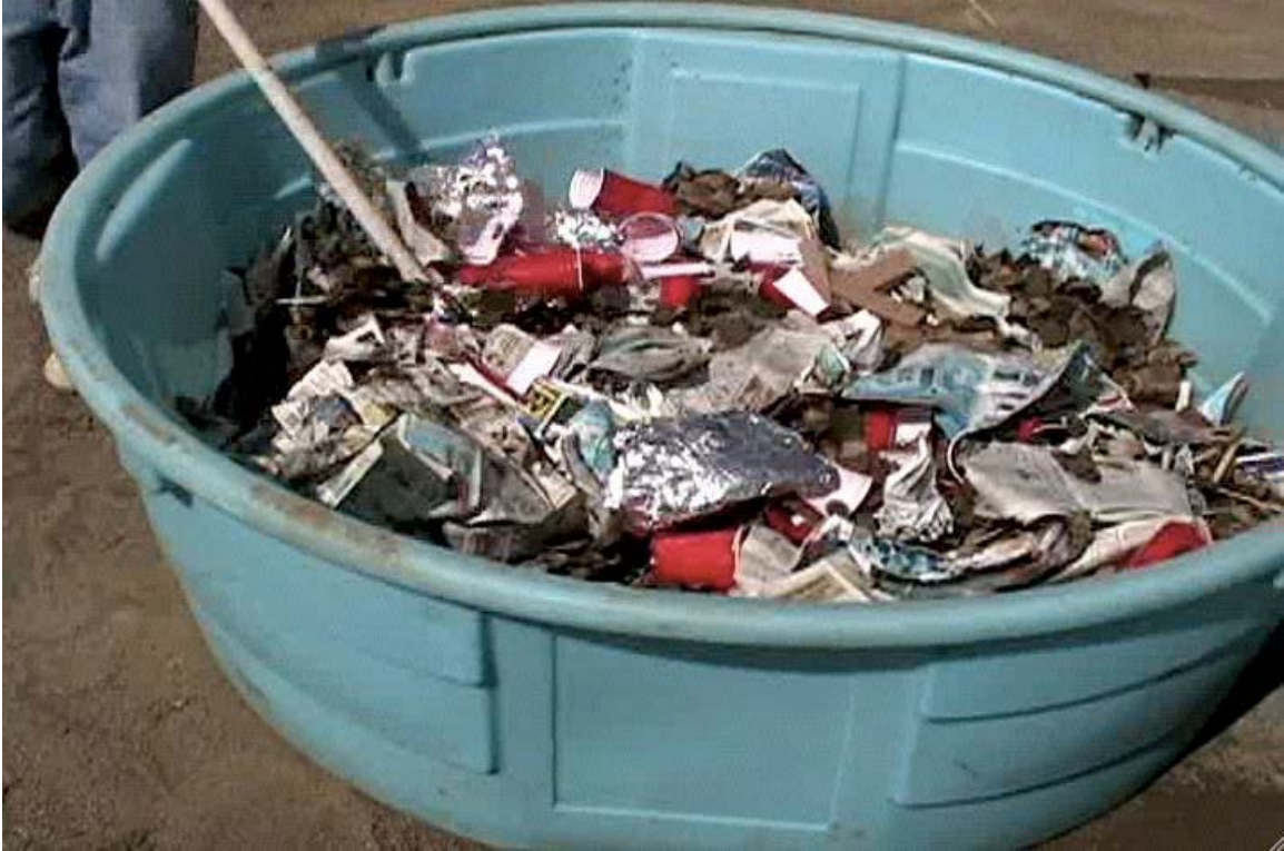
Figure 3.4: Gross solids mix manufactured in the Hydraulics Laboratory.
