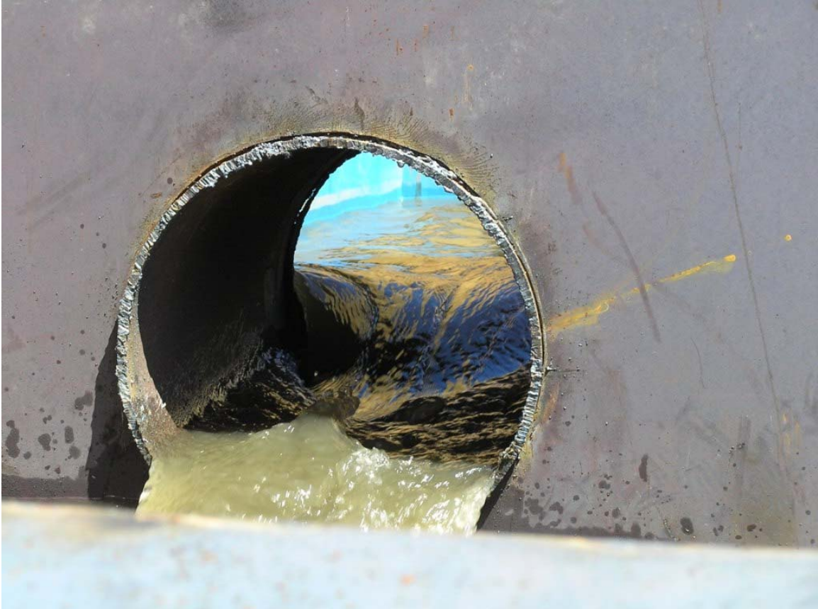
Fig. 6.10: Flow inside inflow pipe for Q=1.85 cfs.
