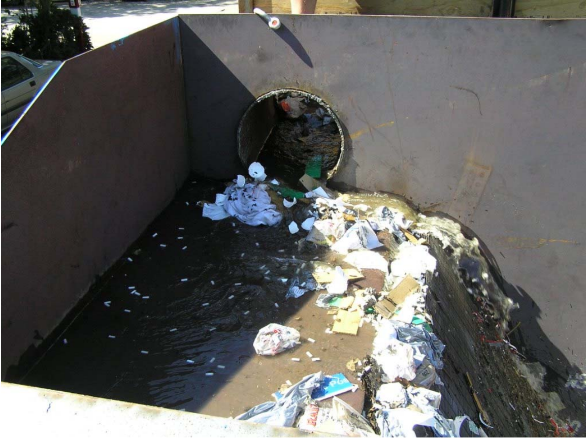
Fig. 6.36: 50% loading at Q=1.1 cfs.
