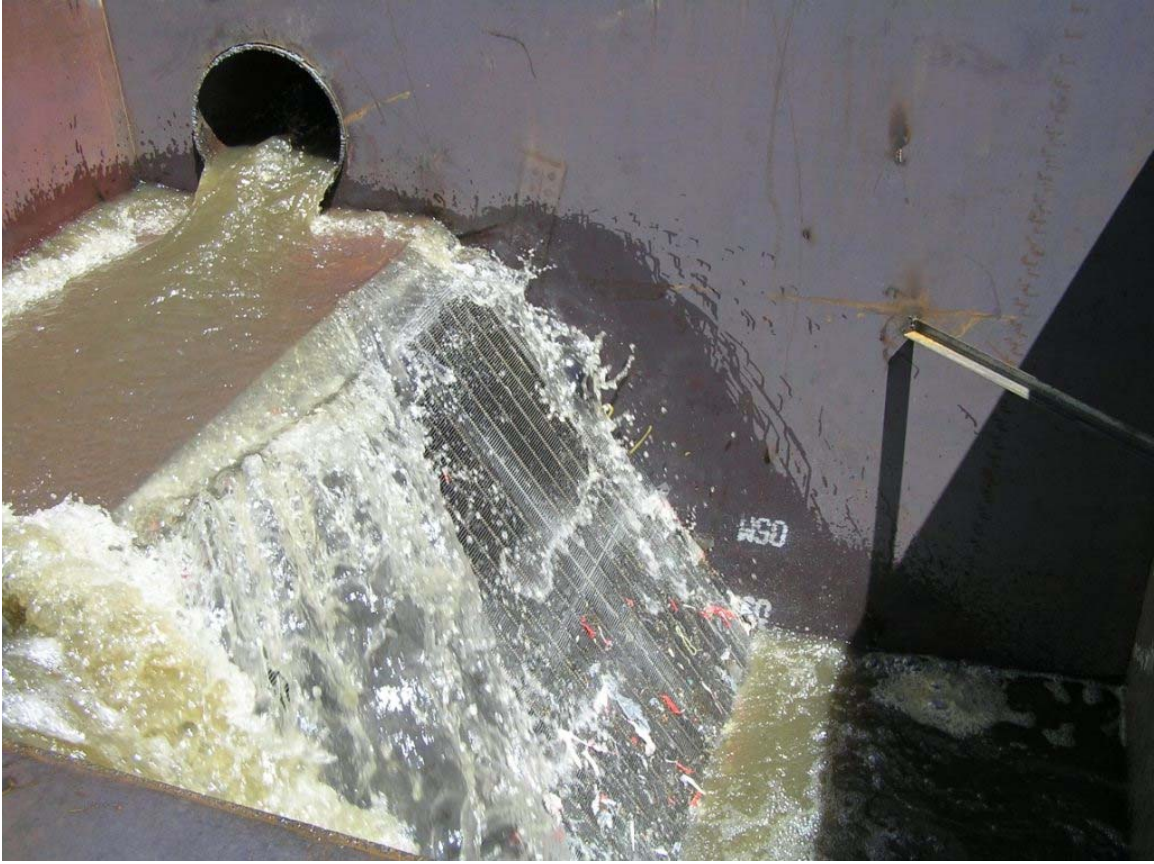
Fig. 6.15: Conditions over screen at Q=2.7 cfs.
