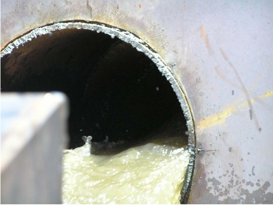
Fig. 6.22: Inlet conditions for Q=6.13 cfs.
