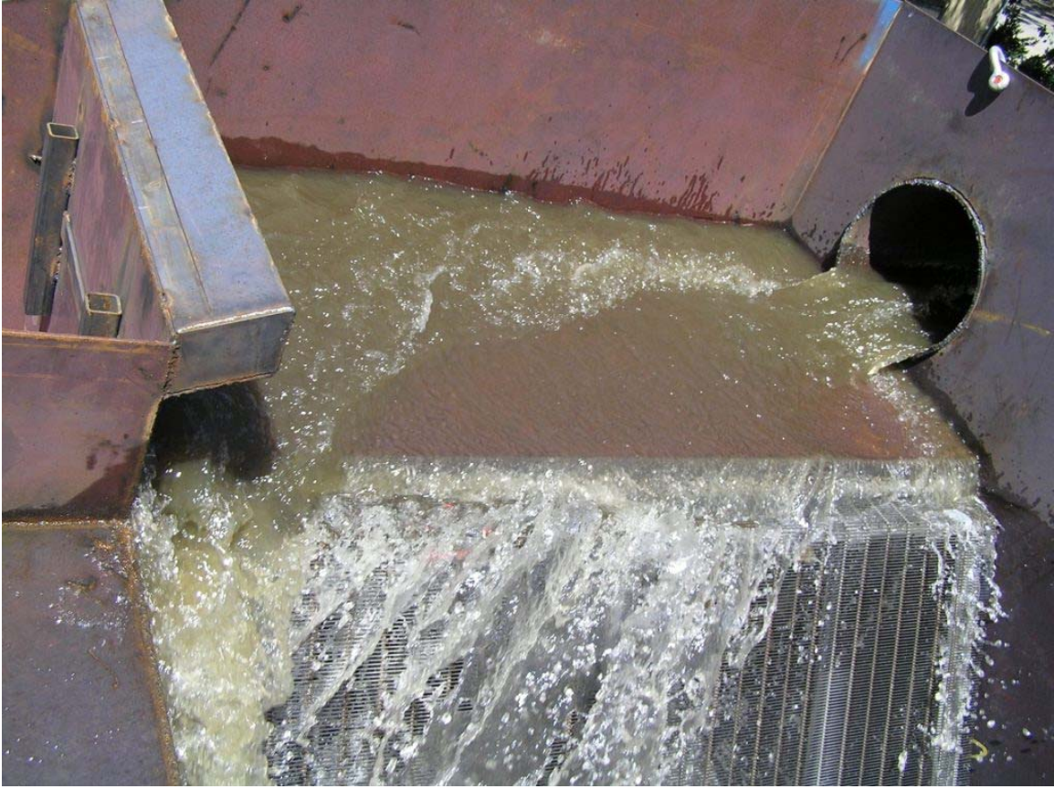
Fig. 6.11: Non-uniform distribution for Q=1.85 cfs.
