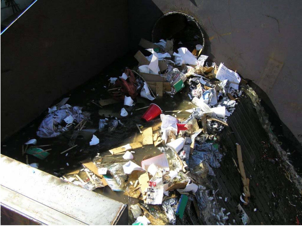
Fig. 6.40: Inflow patterns for Q=1.1 cfs and 90% loading.
