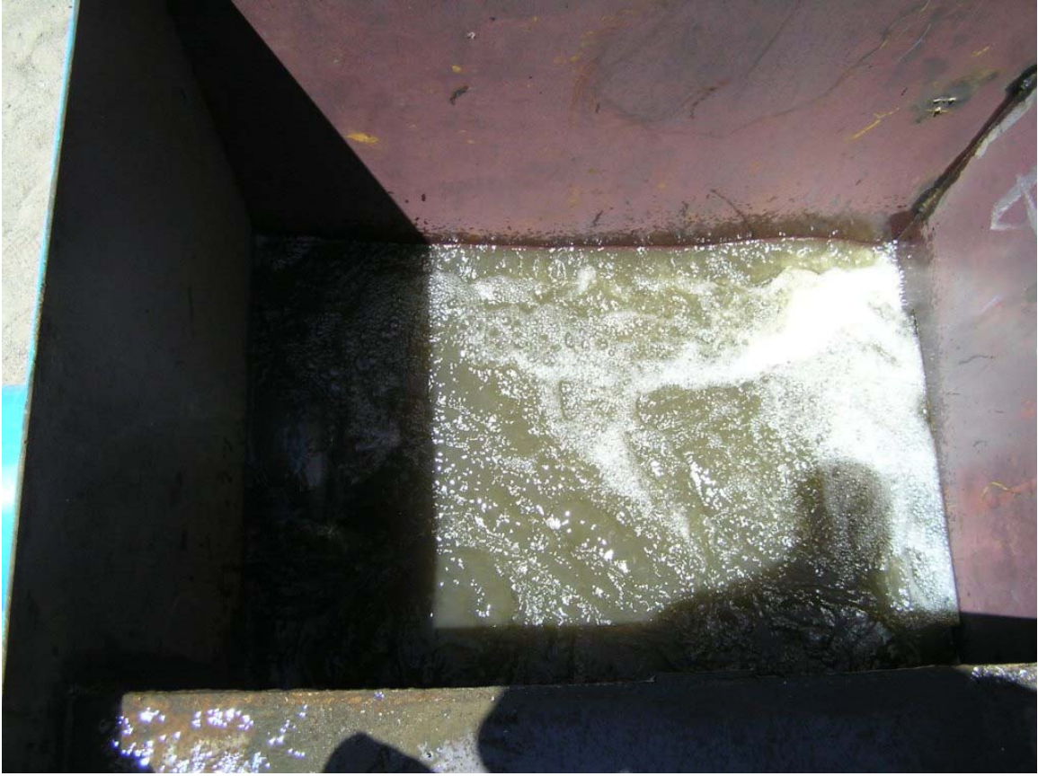
Fig. 6.24: Conditions at outflow for Q=6.13 cfs.
