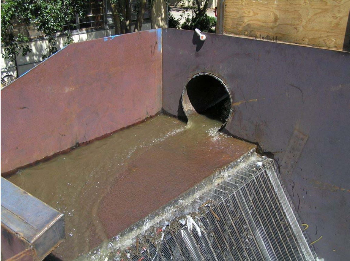
Fig. 6.7: Inflow conditions for Q=0.94 cfs.
