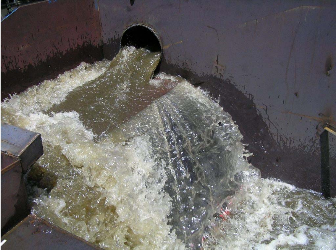
Fig. 6.20: Flow over screens for Q=5.0
