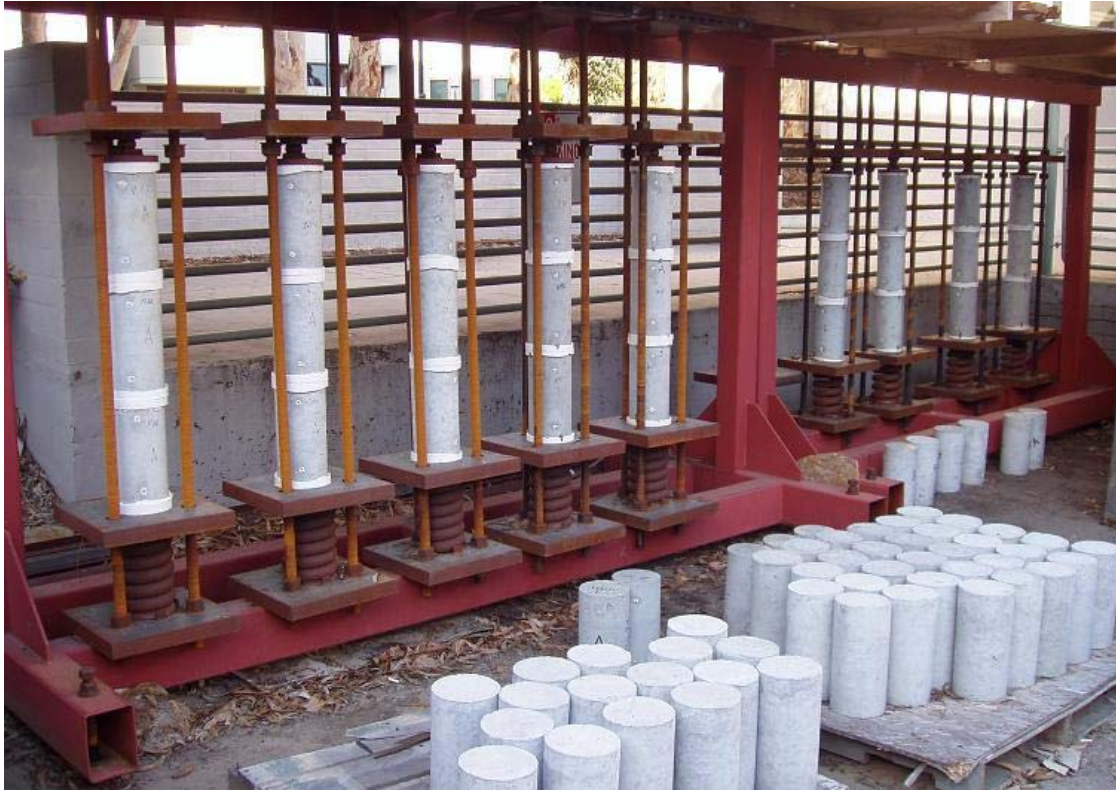
Figure 3.10: All creep test setups.
