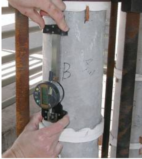
Figure 3.11: Measuring with DEMEC gage.
