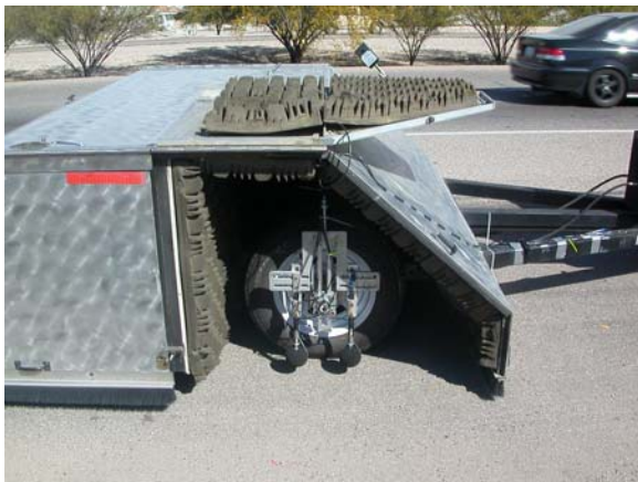
Figure 4: First application of a 2 probe SI method for measuring tire/pavement noise on CPX trailer as developed for ADOT use (July 2003)
