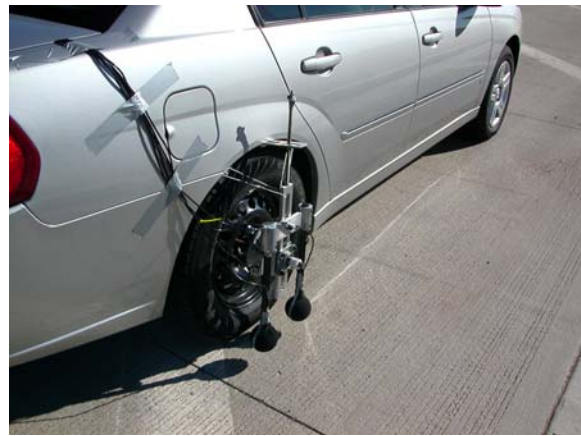
Figure 5: Application of a 2 probe SI method for measuring tire/pavement noise in exposed flow mounted on a test vehicle as used in joint ACPA/Caltrans testing (November 2005)
