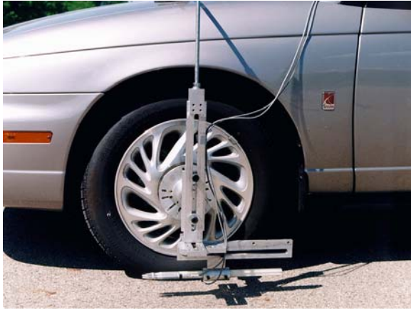
Figure 2: Configuration for SI application to tire/pavement noise measurement on passenger cars for use in quantifying tire noise source levels at the General Motors Proving Ground (Ref. 3)
