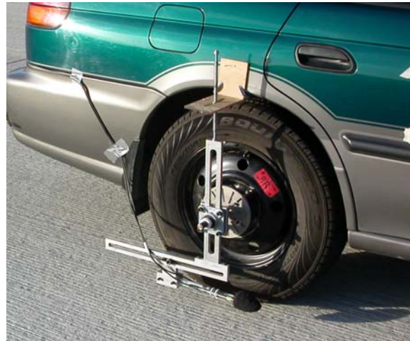
Figure 3: Configuration for SI application to tire/pavement noise measurement for purposes of quantifying highway pavement performance as employed on Caltrans projects starting in 2002
