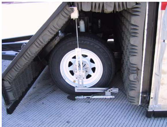
Figure 15: Single probe SI fixture as installed on the ADOT CPX trailer for joint ADOT/Caltrans pavement noise studies (May 2002)
