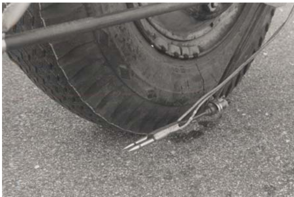
Figure 1: Configuration for first application of SI to tire/pavement noise measurement as used for truck tire noise source identification at General Motors Research (Ref. 2)
