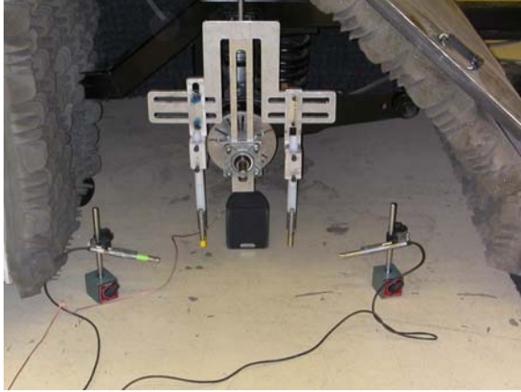
Figure 18: In-lab testing to detect reflections or other effects of CPX 2 probe SI fixture on sound pressure levels received at the CPX microphone locations using a loudspeaker source in July 2003 (measurements made with the ADOT trailer door closed)
