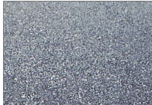
Figure 5: Suitable Surface, Open Graded HMA
