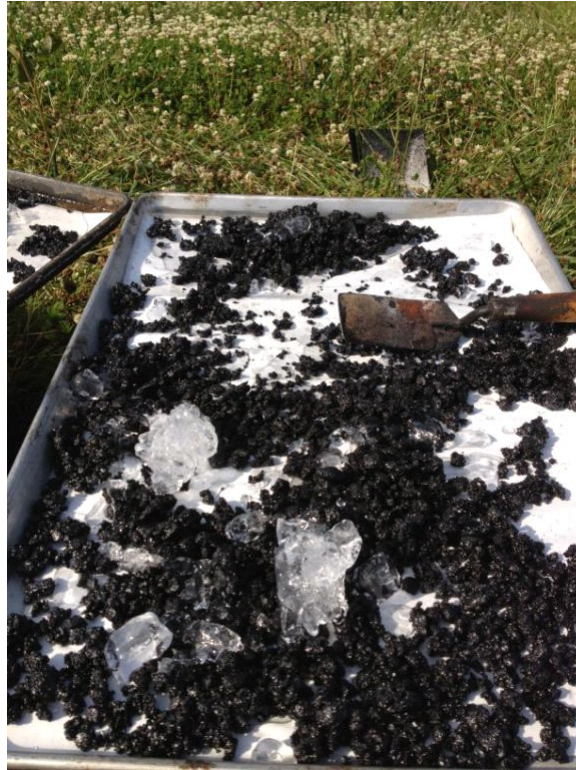
Figure 7: Example of Ice Placed on Field Sample
