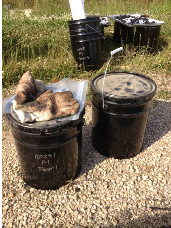
Figure 8: Reheat Samples within Metal Buckets
