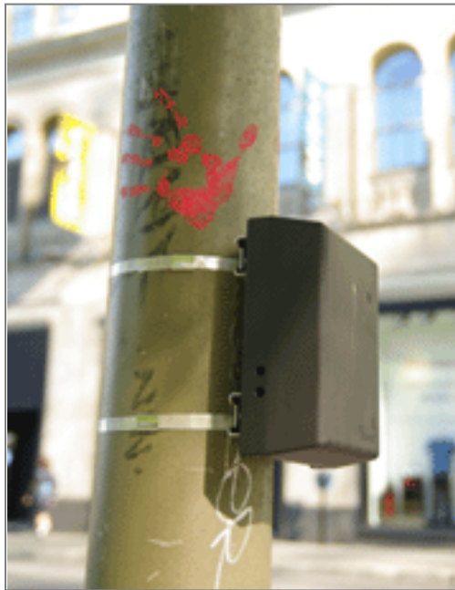
Figure 3.10. EcoCounter Pyroelectric Infrared Sensor ( EcoCounter 2013 )
