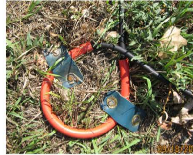
1e. Red Rubber Hose- used to secure MC 2' Red
