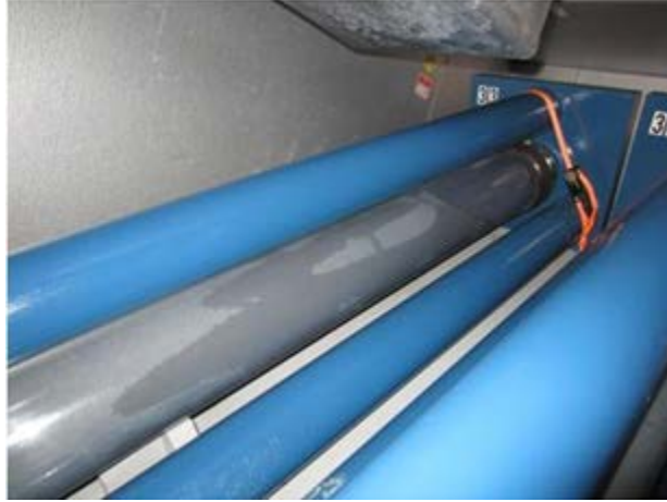
Figure 54. Photo. Multi-strand specimen 1 h after water charging.
