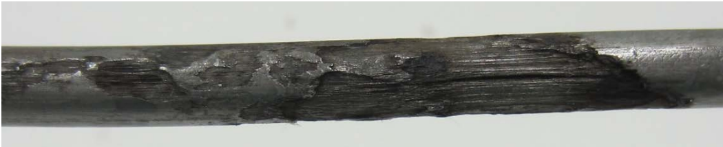
Figure 245. Photo. 0 percent chloride multi-strand specimen at the interface (pit depth = 2–36 mil).
