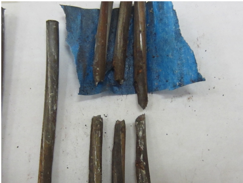
Figure 221. Photo. Close-up view of the broken wires shown in figure 220.
