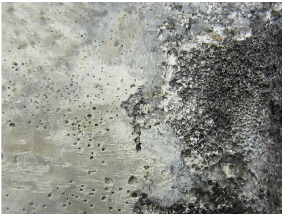
Figure 214. Photo. Close-up plan view of the void/grout interface (top section).
