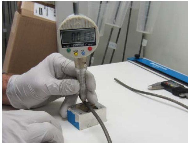
Figure 77. Photo. Pit depth measurement using a digital pit gauge.
