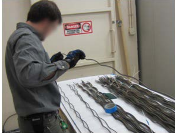
Figure 76. Photo. Cleaning and visual inspection of 7-ft-long unstressed strands.
