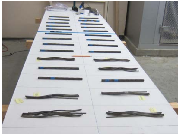
Figure 75. Photo. Several 12-inch-long cut-out segments exhibiting various corrosion conditions.
