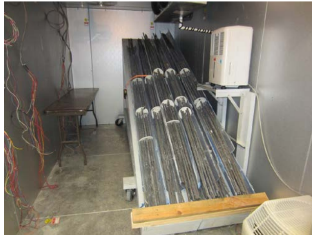
Figure 73. Photo. Storing the retrieved multi-strand samples in a chamber.
