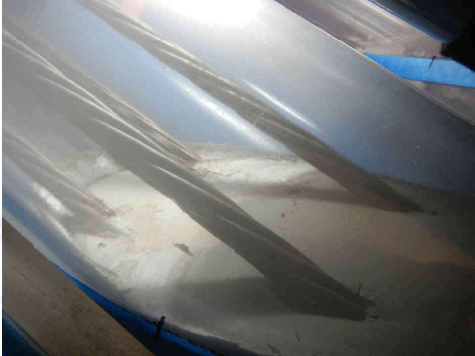
Figure 162. Photo. Void condition of 1.0 percent chloride specimen.
