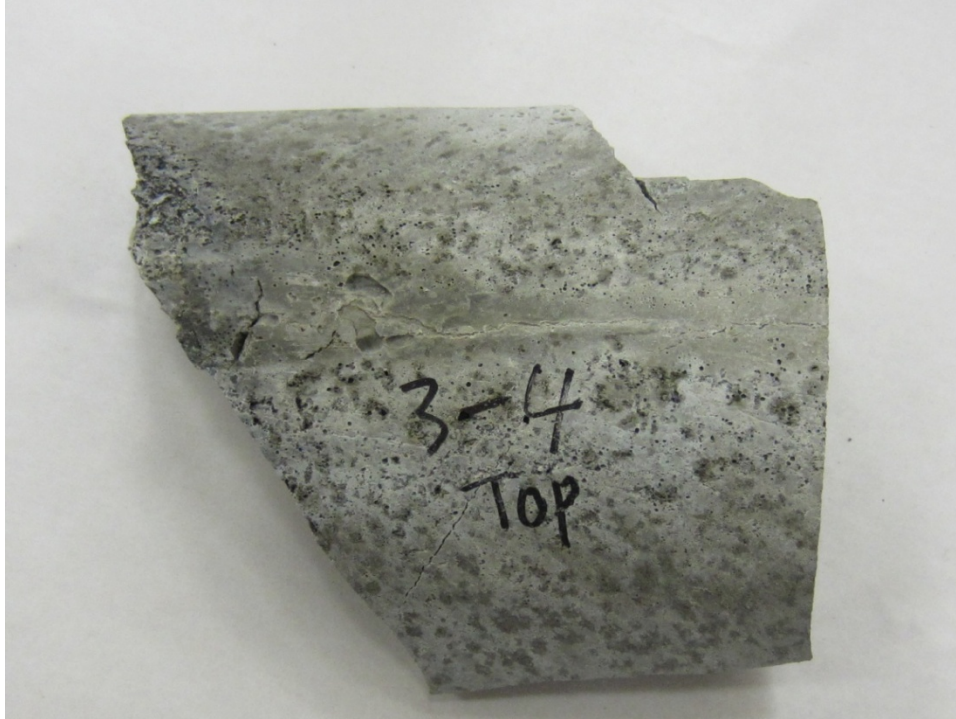
Figure 222. Photo. Top side grout piece exhibiting bleed channel and porous grout removed from 0.4 percent chloride specimen.
