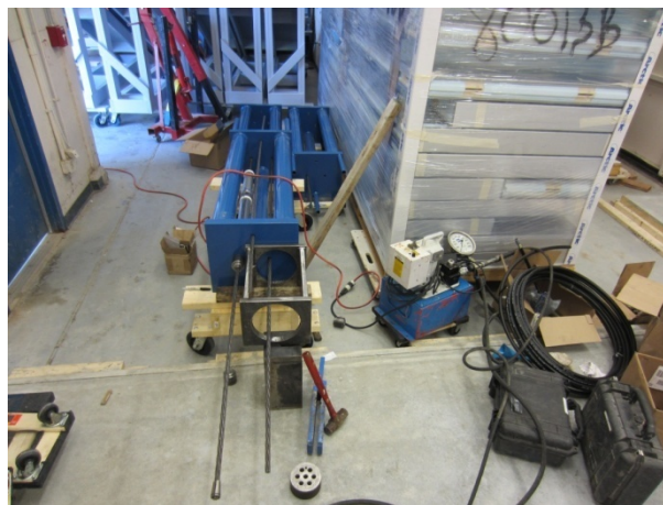
Figure 29. Photo. Stressing of single-strand specimens.
