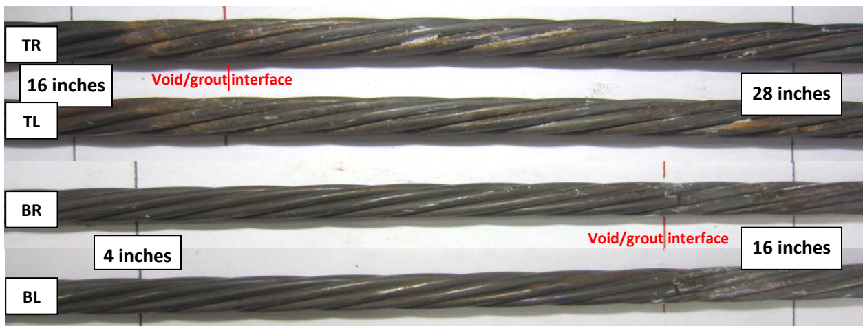
Figure 212. Photo. As-extracted condition of four stressed strands at the void/grout interface of 0.8 percent chloride multi-strand specimen.
