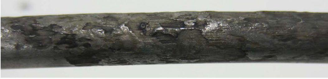
Figure 240. Photo. 0 percent chloride multi-strand specimen at the void/grout interface (pit depth = 2–4 mil).
