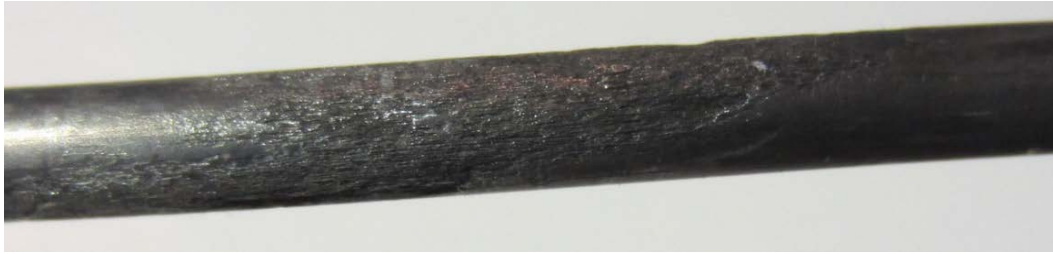
Figure 241. Photo. 0.08 percent chloride multi-strand specimen near the interface (pit depth = 2–10 mil).
