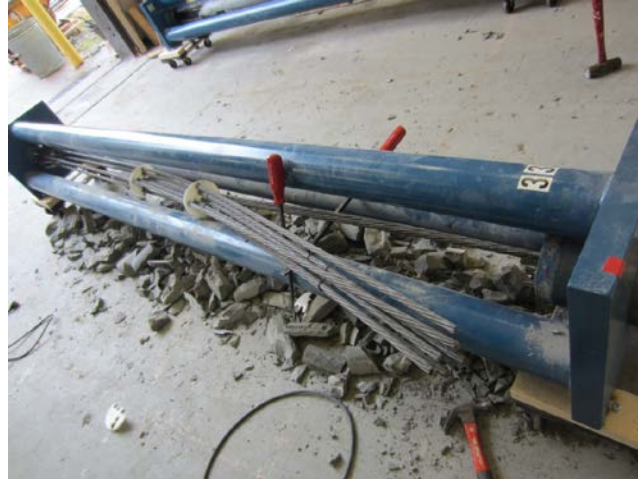
Figure 72. Photo. Extracting a multi-strand bundle from a loading frame.
