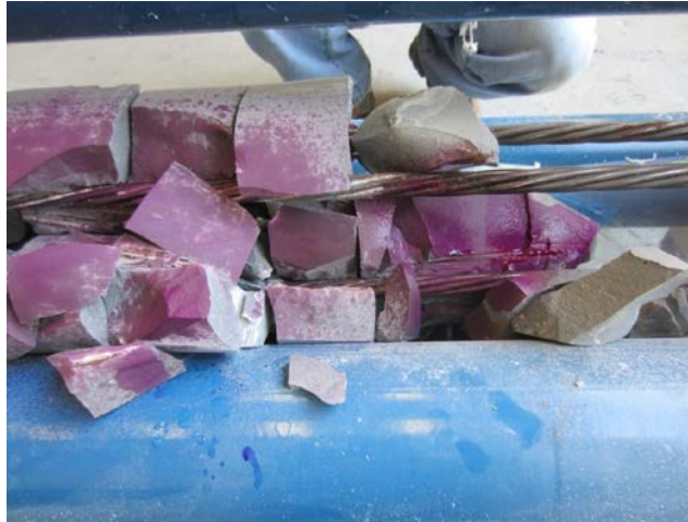
Figure 232. Photo. Carbonation testing results of 0.8 percent chloride multi-strand specimens.
