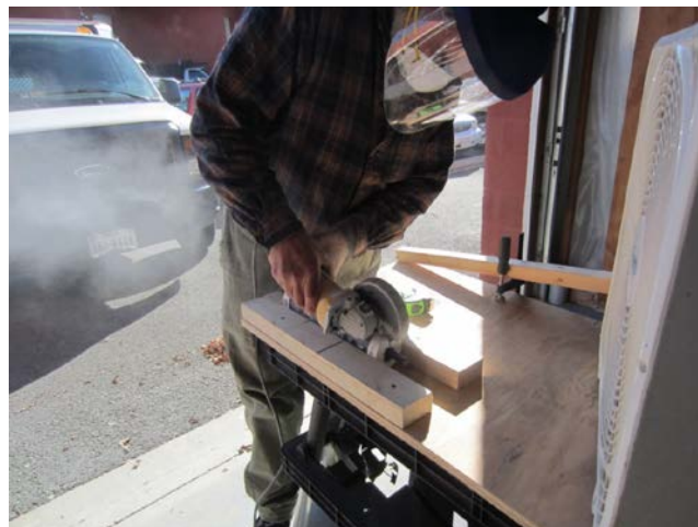
Figure 60. Photo. Splitting a single-strand specimen using a circular saw.
