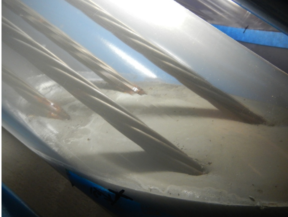
Figure 160. Photo. Void condition of 0.6 percent chloride specimen.
