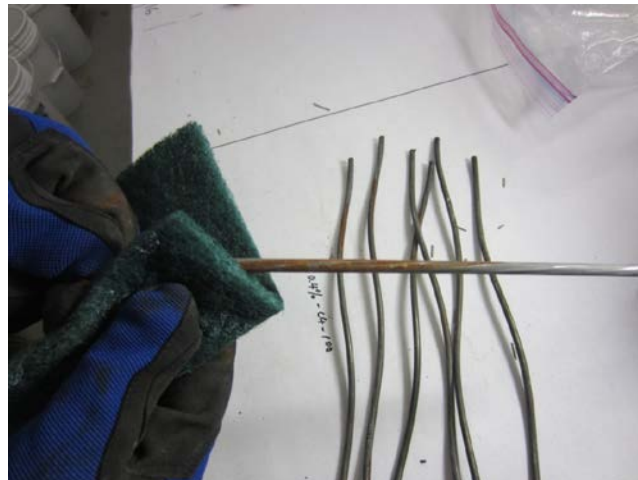
Figure 64. Photo. Cleaning individual wires using a scrubbing pad.
