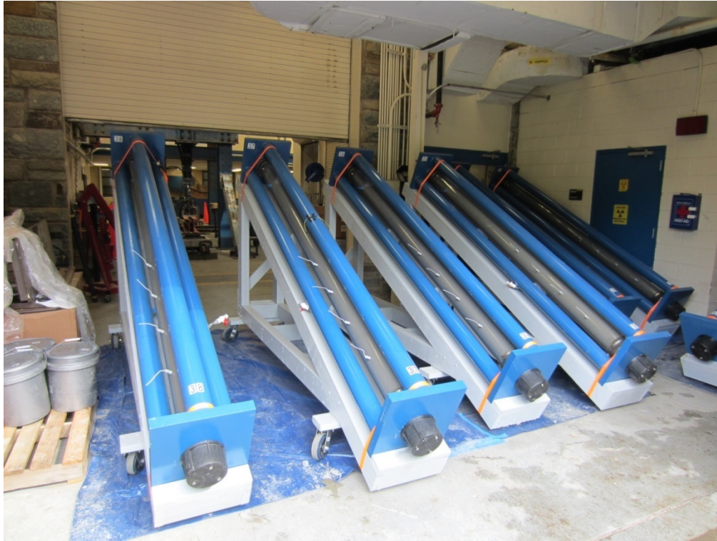
Figure 38. Photo. Fully assembled multi-strand specimens.
