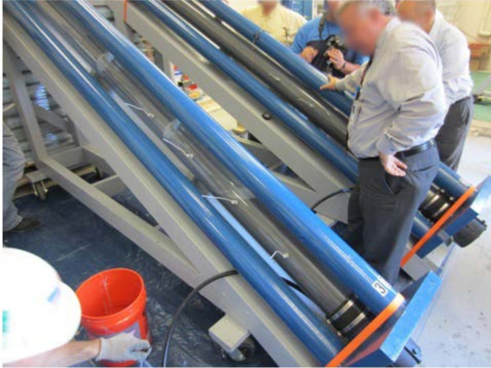
Figure 39. Photo. Grout pumping into a multi-strand specimen.
