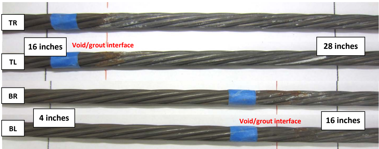
Figure 210. Photo. As-extracted condition of four stressed strands near the void/grout interface of 0.08 percent chloride multi-strand specimen.
