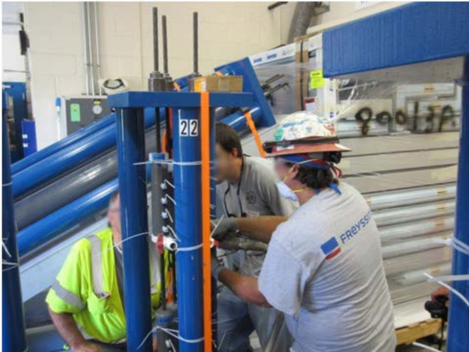
Figure 33. Photo. Grout pumping into a single-strand specimen.
