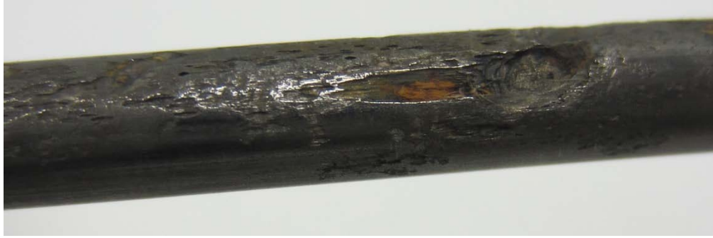
Figure 244. Photo. 1.0 percent chloride multi-strand specimen in the grout (pit depth = 2–23 mil).
