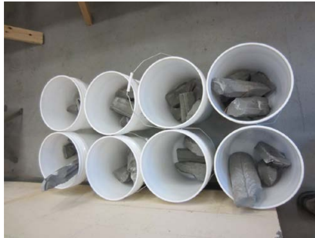
Figure 70. Photo. Retrieved grout pieces from multi-strand specimens.
