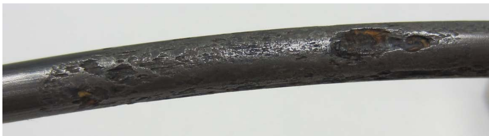
Figure 243. Photo. Stressed and voided 1.0 percent chloride single-strand specimen (pit depth = 2–18 mil).
