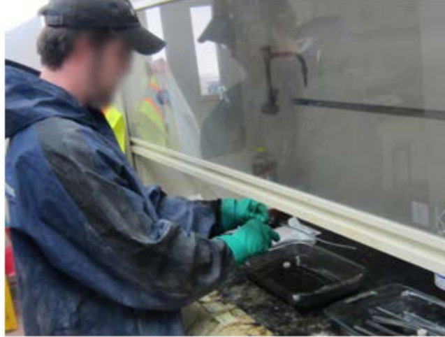
Figure 65. Photo. Acid cleaning of moderately to severely corroded wires.
