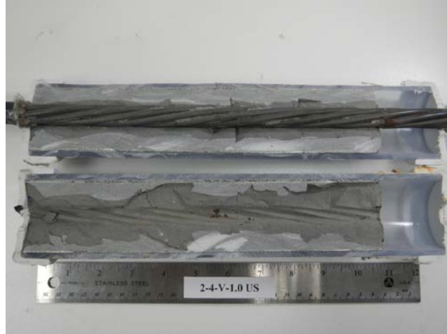
Figure 61. Photo. Single-strand specimen longitudinally cut in half.
