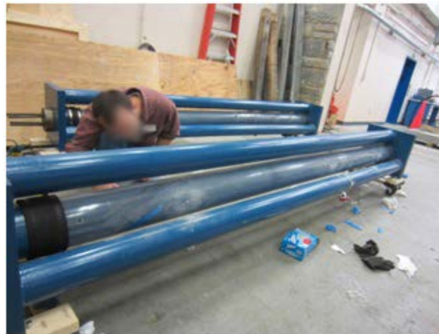
Figure 67. Photo. Grout powder sampling for chloride analysis from a multi-strand specimen.
