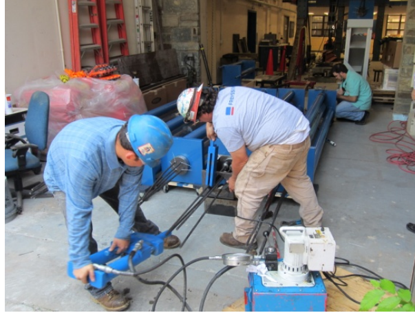
Figure 30. Photo. Stressing of multi-strand specimens.
