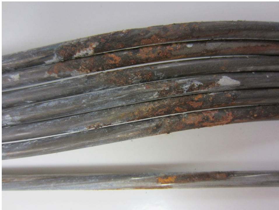
Figure 218. Photo. As-extracted condition of another stressed segment passed through the contaminated void/grout interface of 0 percent chloride multi-strand specimen.
