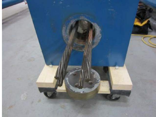
Figure 66. Photo. Removal of the upper anchor bearing plate of a multi-strand specimen.
