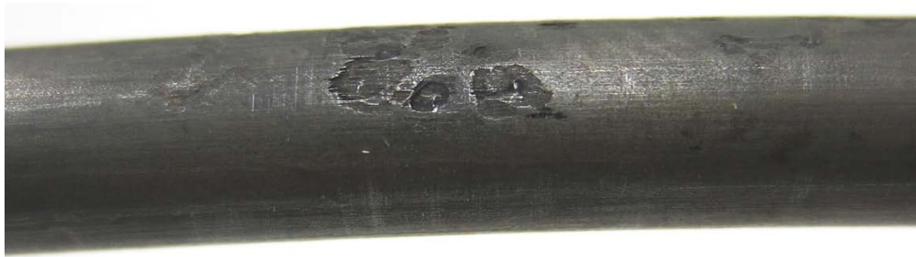
Figure 238. Photo. Stressed and fully grouted 0.8 percent chloride single-strand specimen (pit depth ~2 mil).
