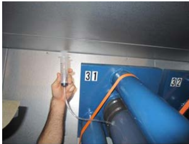
Figure 52. Photo. Water charging into a multi-strand specimen.
