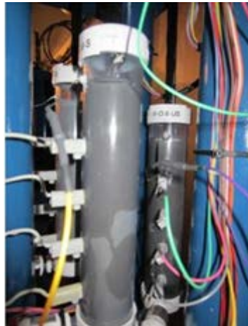
Figure 55. Photo. Single-strand specimen 1 h after water charging.
