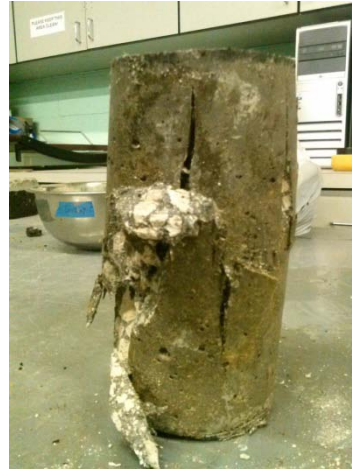
(b) Fiber reinforced concrete (M08)
