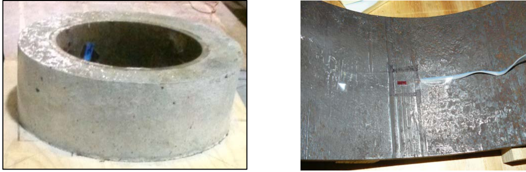
Figure 3.12 - Restrained shrinkage specimen and strain gages
