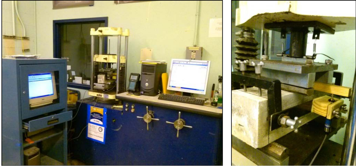
Figure 3.6 - Flexural test setup
