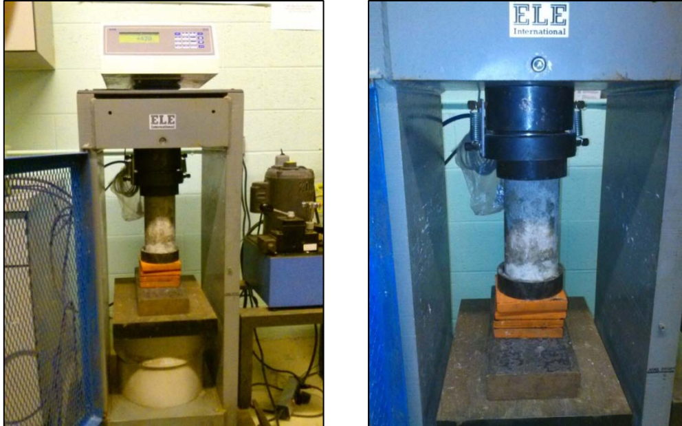
Figure 3.5 - Compression test setup
