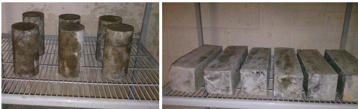
Figure 3.3 - Specimen surface drying before testing
