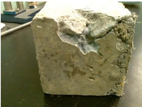
(a) pockets due to fiber balling
