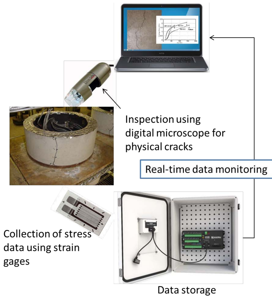
Figure 3.13 - Schematic of restrained shrinkage test
