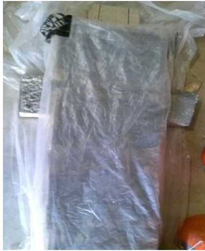
Figure 3.4 - Specimen protection and curing
