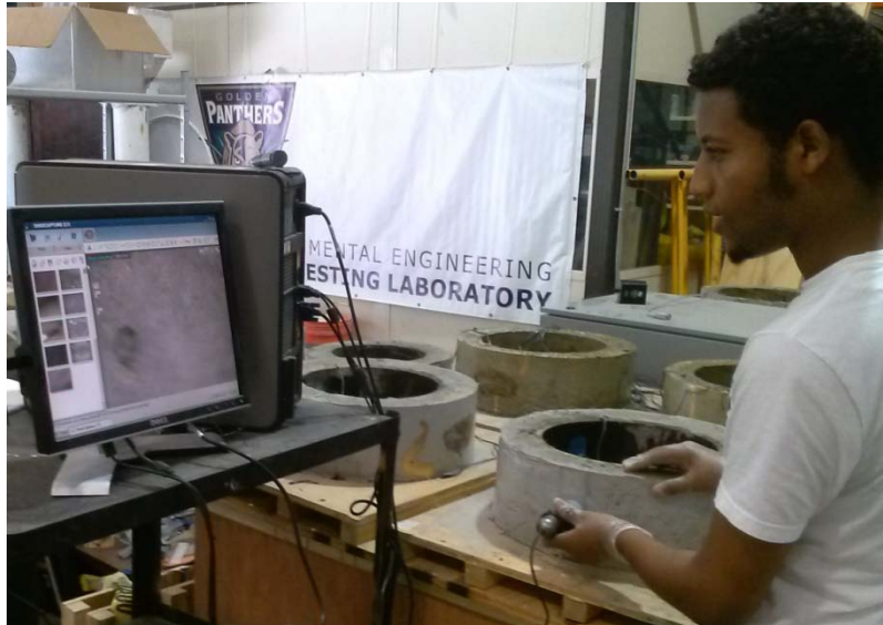
Figure 3.14 - Inspection of physical cracks
