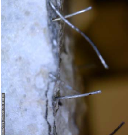
Figure 4.7 - Pull out of steel fibers. The holes on the right indicate pull out locations
