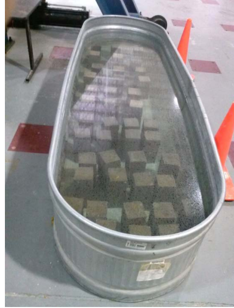
Figure 3.4 - Specimen protection and curing
