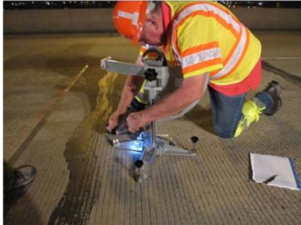
Fig 3.11 CDOT engineer conducting a skid resistance test
