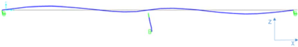
Figure 34. Mode 4 for the modified bridge. Note the lateral movement apparent at the right end of the bridge due to a roller fixity rather than a pinned fixity in the x direction.
