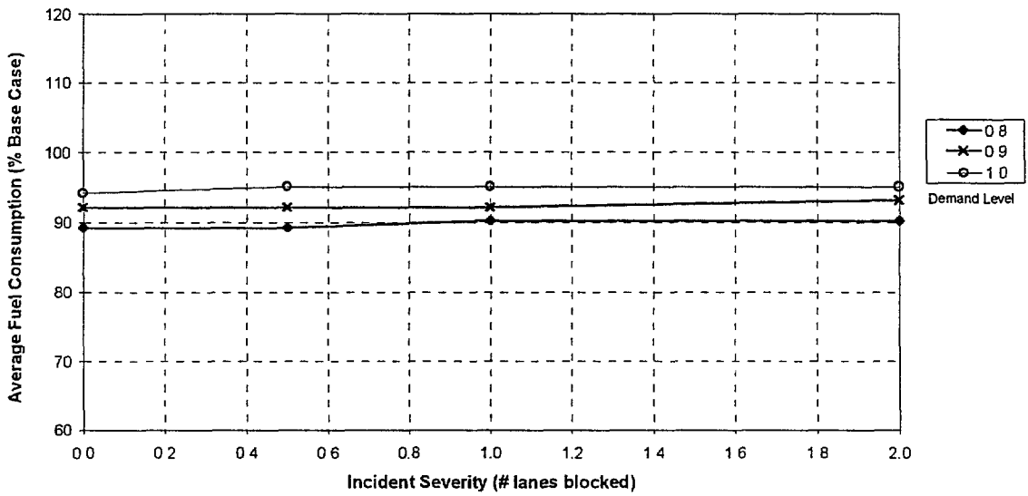
Figure B-43. Variation in average fuel consumption as a function of incident severity and demand level (20% LMP)
