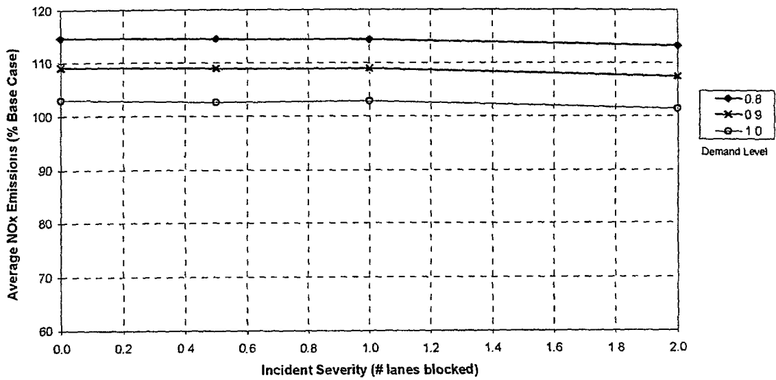
Figure B-79. Variation in average NO x emissions as a function of incident severity and demand level (20% LMP)
