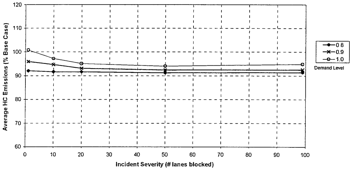
Figure B-49. Variation in average HC emissions as a function of LMP and demand level (No incident)
