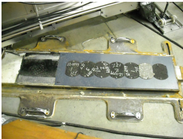
Figure 4. Set of Briquettes Installed in Testing Frame: before ( left ) and after ( right ) being tested under the MMLS3
