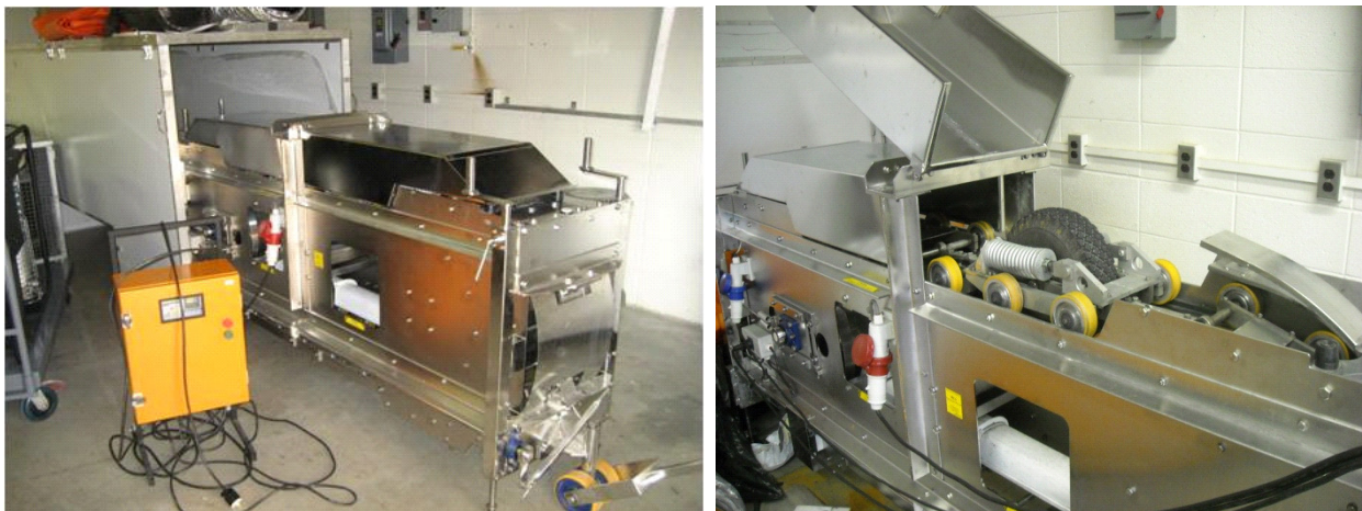
Figure 1. Mobile Model Load Simulator (MMLS3) with Environmental Chamber Mounted (left)
