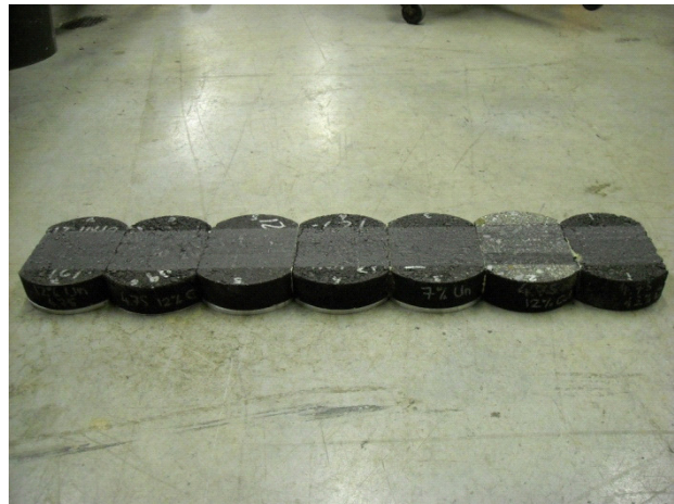
Figure 4. Set of Briquettes Installed in Testing Frame: before ( left ) and after ( right ) being tested under the MMLS3
