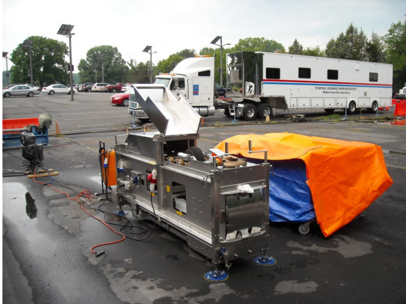
Figure 2. Testing for Rutting of SM-4.75 Mixture at Turner-Fairbank Highway Research Center. Cooling/heating unit pictured to right.
