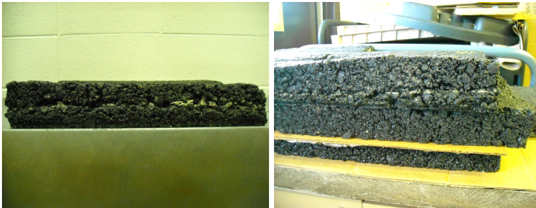
Figure 10. Debonding and Heaving in SM-12.5D HR Mixture During Rutting Tests at 147° F (64° C)
