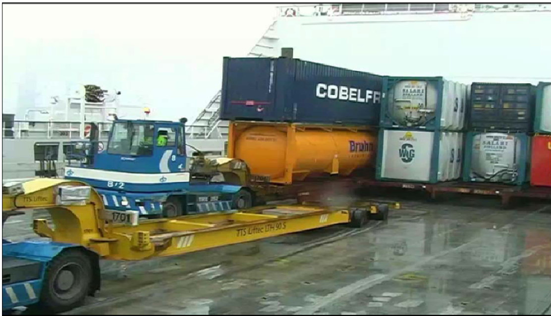
Figure 11 The cassette system (Source: TTS, 2013)
