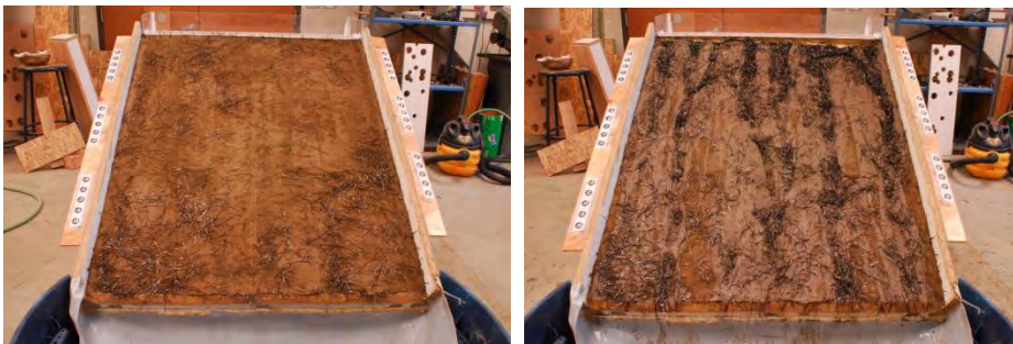
Fig. A-26: Before and After Pictures of 6% w + 4% EVK + 0.5% GF – Test 2
