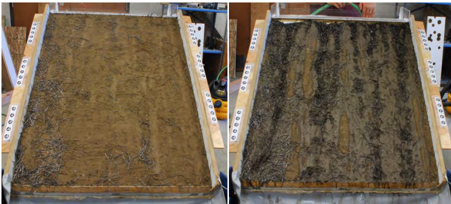
Fig. A-23: Before and After Pictures of 6% w + 2% SS + 0.5% GF – Test 1
