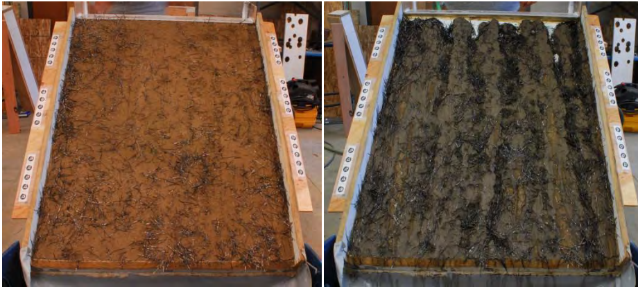
Fig. A-21: Before and After Pictures of 6% w + 0.5% GF – Test 1
