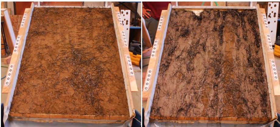
Fig. A-25: Before and After Pictures of 6% w + 4% EVK + 0.5% GF – Test 1
