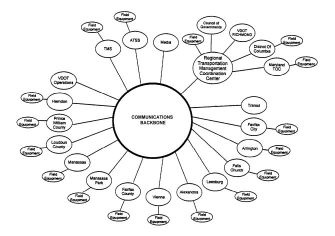
Figure 5.2 - Peer to Peer with Centralized Coordination Architecture
