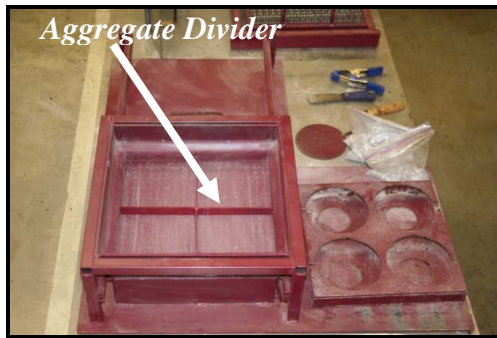
a) Placement of Aggregate Divider
