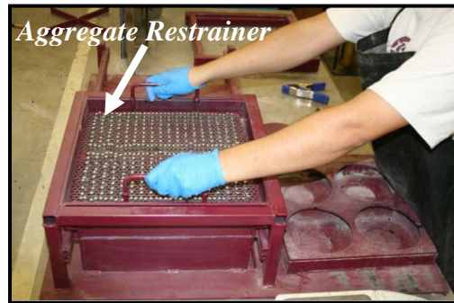
d) Placement of Aggregate Restrainer
