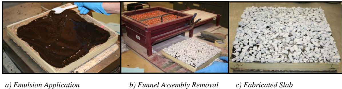
Figure 4.11. Specimen Fabrication Procedure - Slabs
