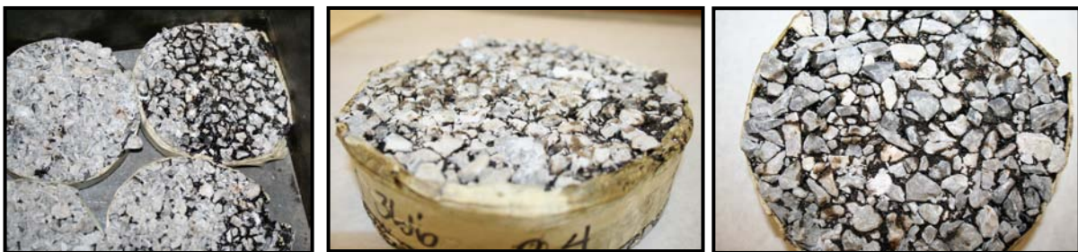
Figure 4.14. Example Photographs of Specimens Damaged During LAC Embedment
