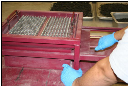
e) Aggregate Spread on LTP Specimens
