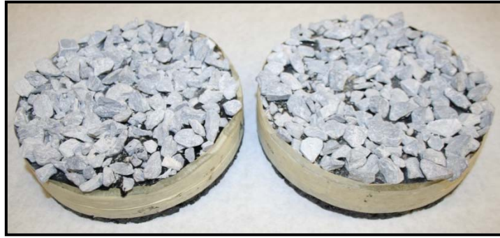
Figure 6.11. Representative Laboratory Fabricated Size 7 Specimens Pre-Embedment
