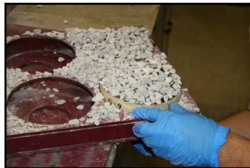
h) Removal of Fabricated Specimen
