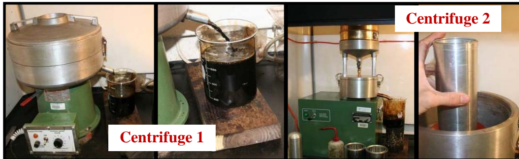
Figure 4.6. Asphalt Extraction Equipment
