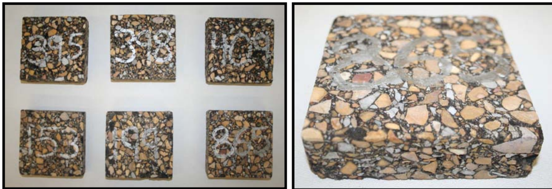
Figure 3.3. Blocks Sawn From Field Aged Pavement for G_{mb} Measurement
