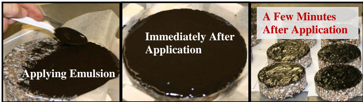
Figure 4.1. Applying Emulsion to Cores
