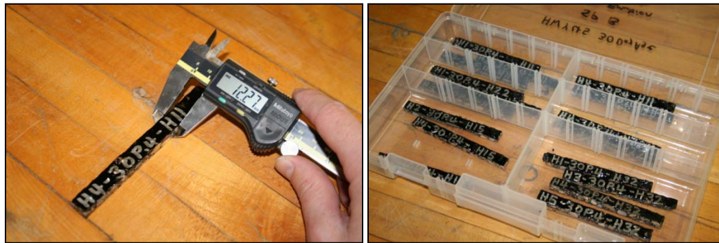
a) Mixture Beam Measuring
