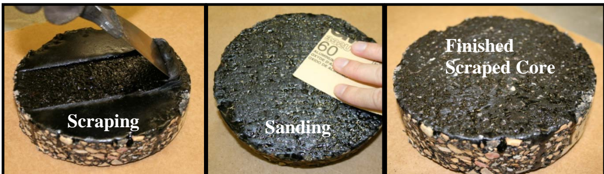
Figure 4.3. Scraping Emulsion Treated Core
