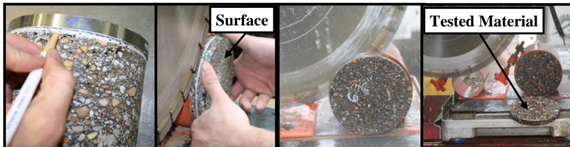
Figure 4.5. Slicing Cores for Viscosity Testing-Untreated Core Shown
