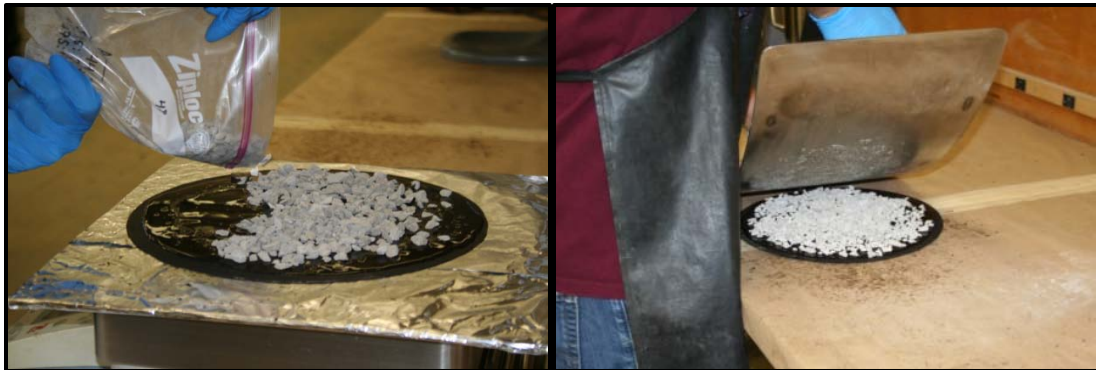
c) Aggregate Spreading d) Aggregate Compaction
