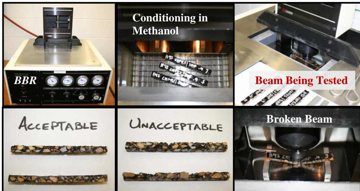
Figure 4.18. Bending Beam Rheometer Testing
