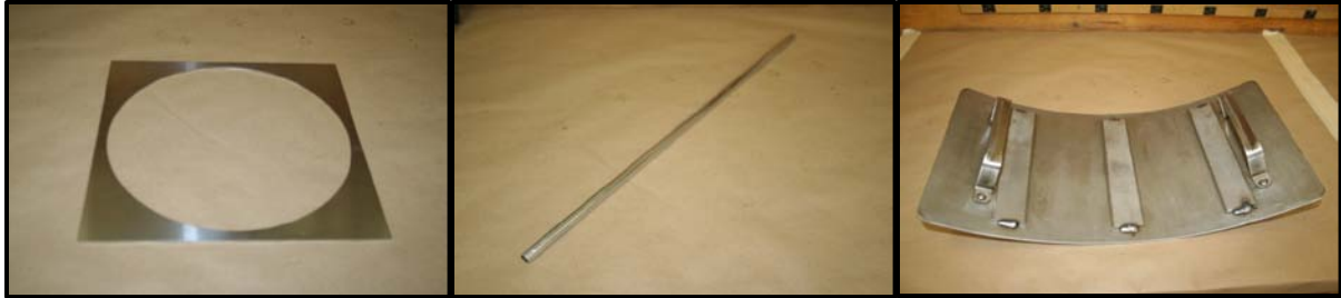
a) Strike-off Template b) Strike-off Rod c) Sweep Test Compactor Figure 4.15. ASTM D7000 Specimen Preparation Equipment
