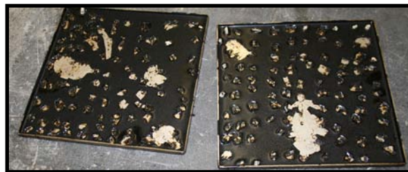
Figure 8.1. Vialit Specification Trays After Testing
