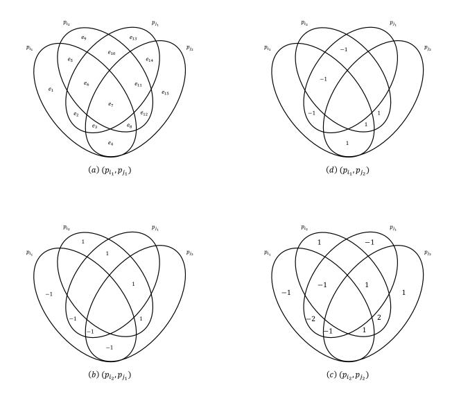
Figure 2.2: Change in the link flows in a simple closed cycle of length 4
