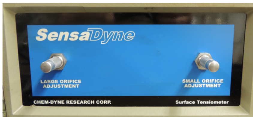
Figure 3.2. Metering valves used to adjust the bubble rate in the large and small orifice
