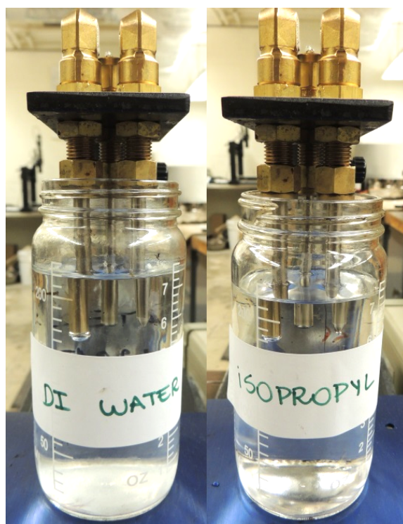
Figure 3.3. Two different liquids are used to calibrate the device to measure surface tension
