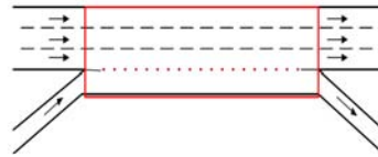
(b) Modeling weaving segments with an auxiliary lane using HCM weaving procedures
