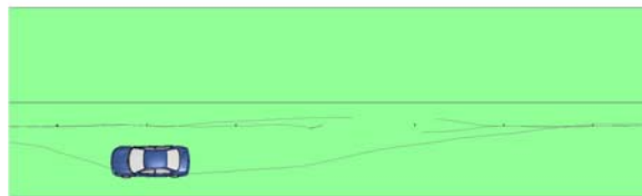
Fig. 3.28: Back-side impact by Dodge Neon at 20° and 65 mph for the first design of Retrofit Option 1.
