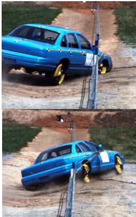
Fig. 2.1: A sedan on its way of penetrating under a cable barrier in a crash test (WSDOT 2006).
