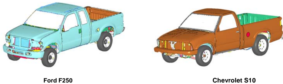
Fig. 3.8: Two NCAC FE models of pickup trucks.
