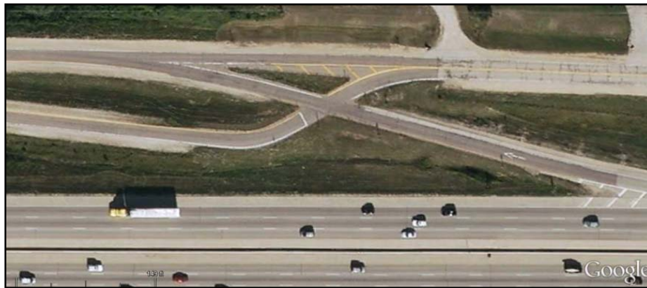
Figure 3-17. Scissors channelization (Image: Google Earth).
