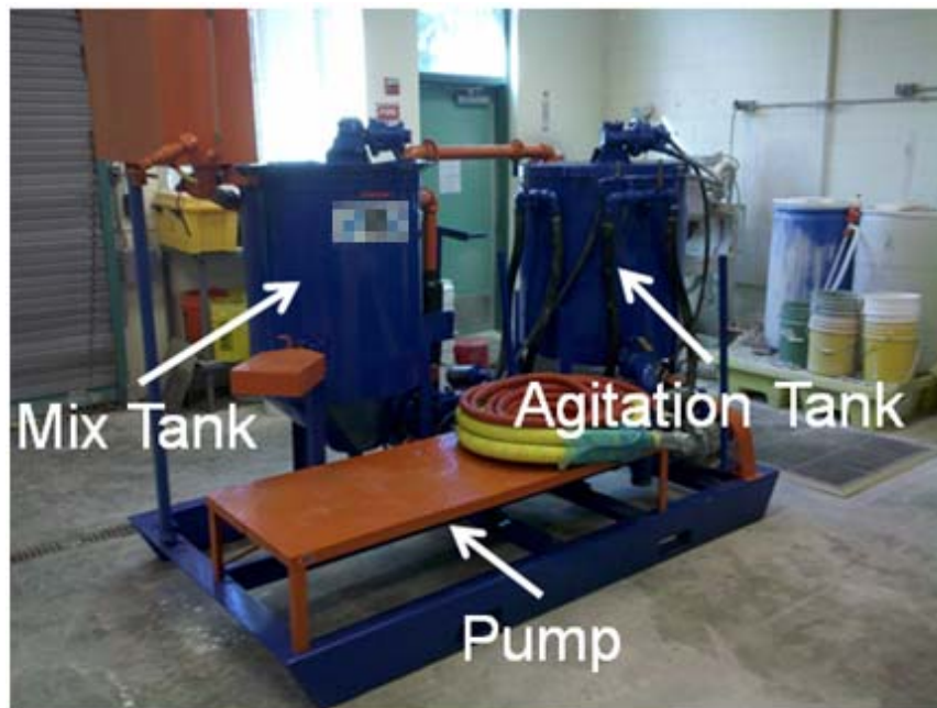
Figure 6—Colloidal grout plant with various parts labeled
