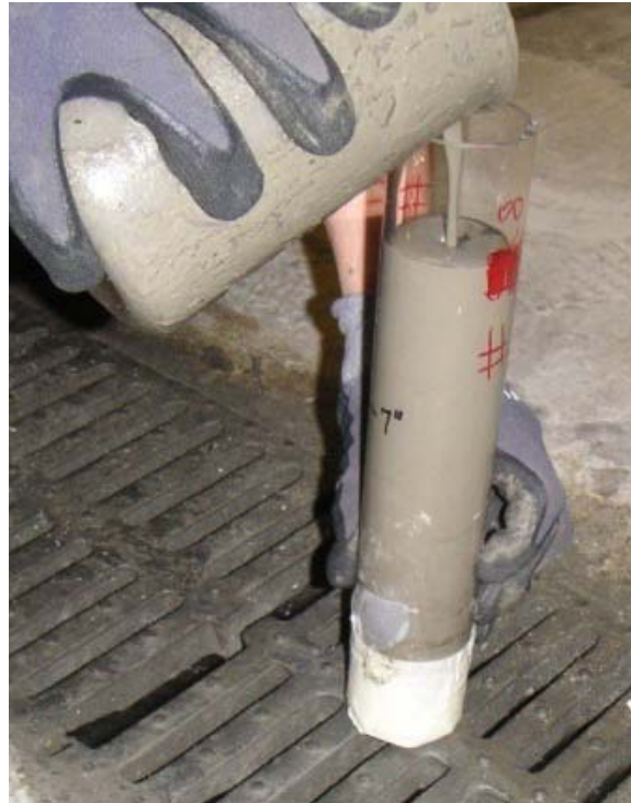
Figure 30—Pouring grout into cylinder for sedimentation test
