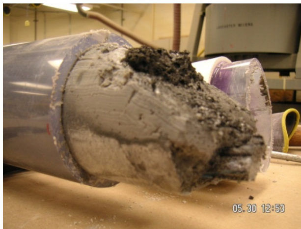
Figure 58—Soft grout and black material found in tubes injected with PT4-2 mixed at 1.15-MWD
