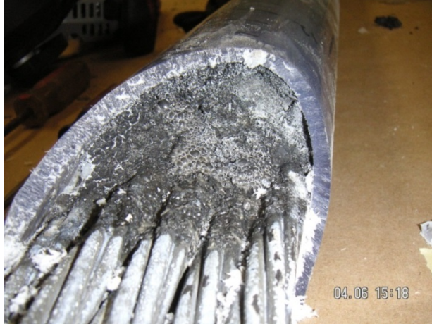
Figure 56—Grout containing air bubbles found at top of tubes containing PT4-1 mixed at MWD
