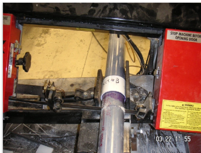
Figure 12—Saw-cut tubes for sampling
