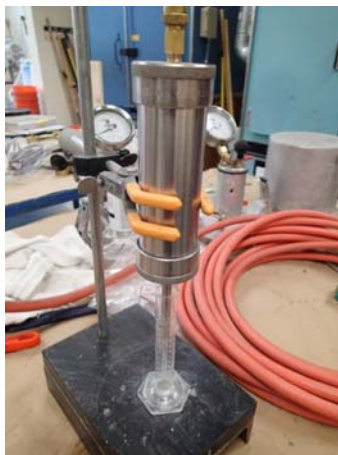
Figure 29—Pressure bleed test setup used during MITT
