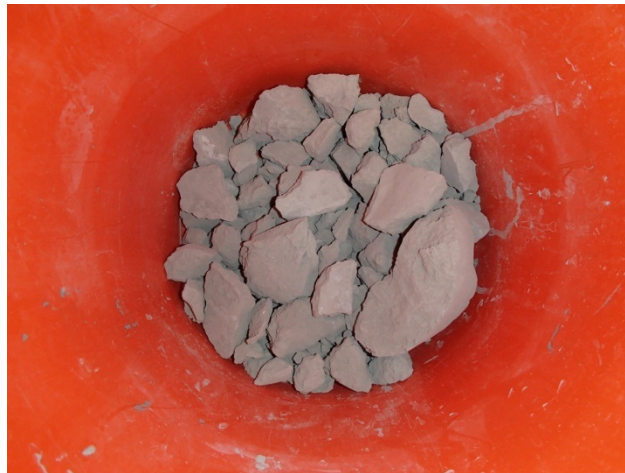
Figure 93—Pre-hydrated grout chunks removed before mixing
