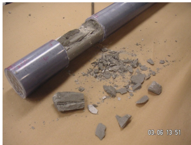
Figure 14—Grout sample removed with chisel
