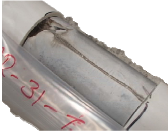
Figure 115—Segregation canal at top of cross-section
