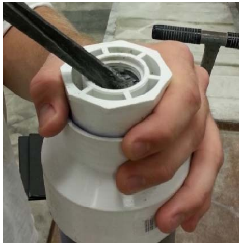
Figure 59—Soft grout found at top of constricted tube containing PT4-2 several months after injection
