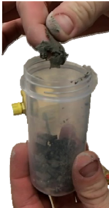
Figure 107—Moist clay like soft grout with darker coloration
