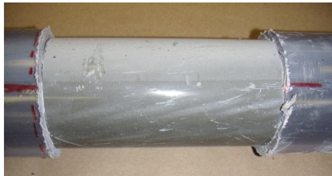
Figure 55—Surface of PT4-1 at MWD. Top half is lighter than bottom half
