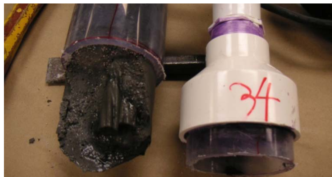
Figure 53—Grout at top of tube when PT2-2 at 1.15-MWD
