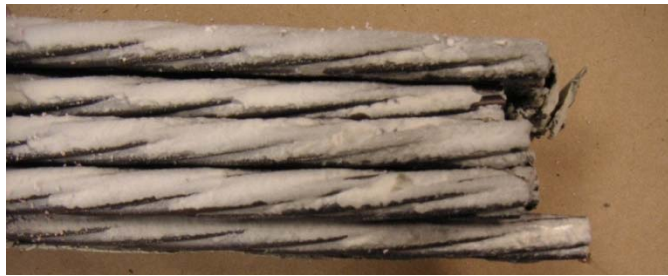
Figure 62—Hard, white material coating strands in tube injected with material C675
