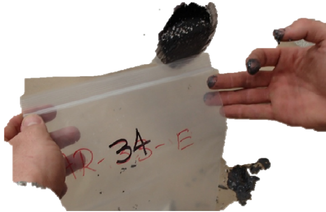
Figure 108—PT4-6 Soft Grout
