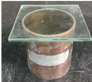
Figure 27—Unit weight used to determine grout density
