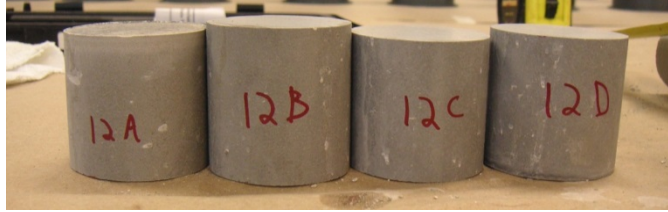
Figure 32—Sedimentation cylinder cut into 4 approximately equal pieces
