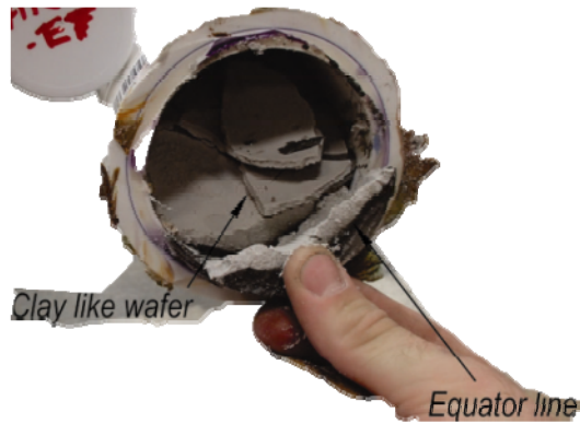
Figure 118—Equator line separating hard cement from soft grout
