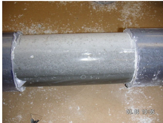
Figure 13—Tube wall removed for sampling
