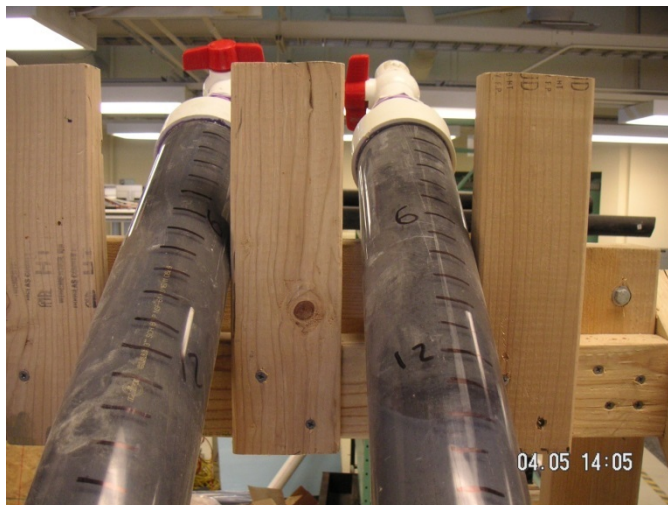
Figure 64—Opaque PVC fittings used on end of inclined tubes
