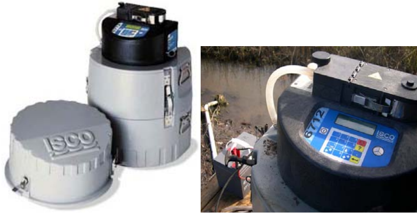
FIGURE 4. Pictures of the Teledyne ISCO 6712 Portable Sampler purchased to be deployed at the Stormwater Demonstration Facility
