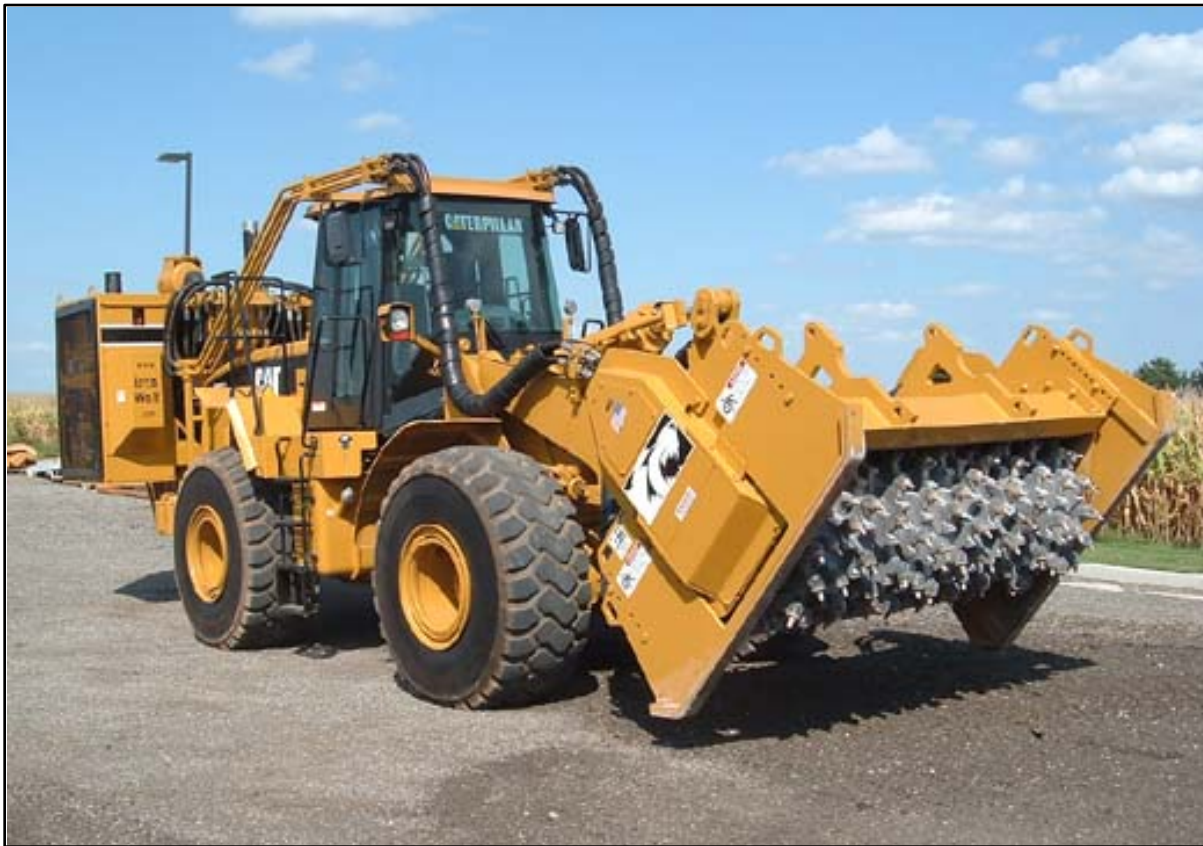
Figure 27. Equipment Used to Mix Soil with Lime.
