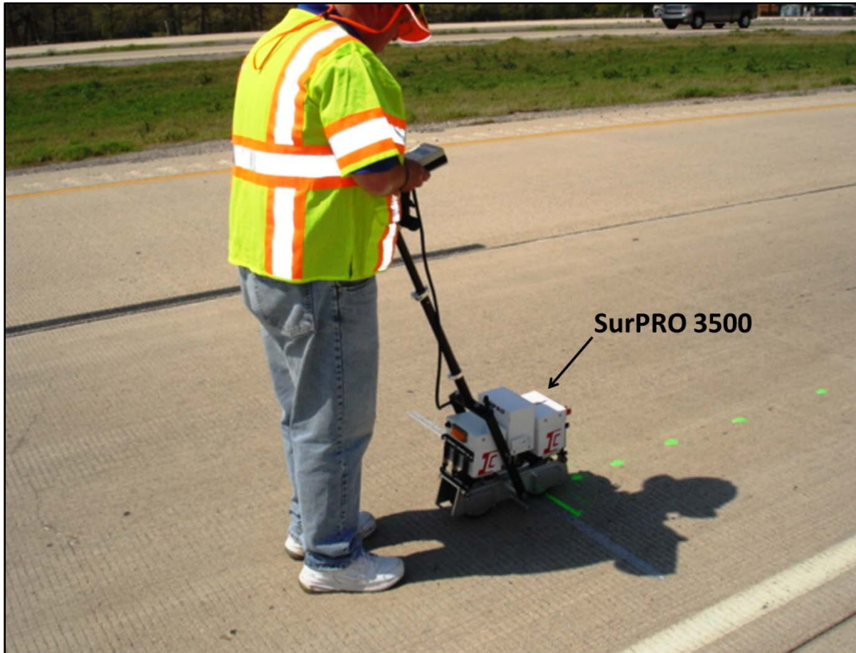
Figure 57. Instrument Used to Measure Reference Profiles.
