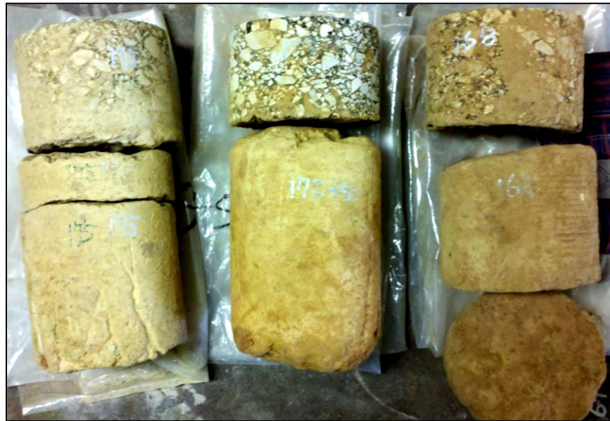
Figure 23. Subgrade Core Samples from FM 1938.
