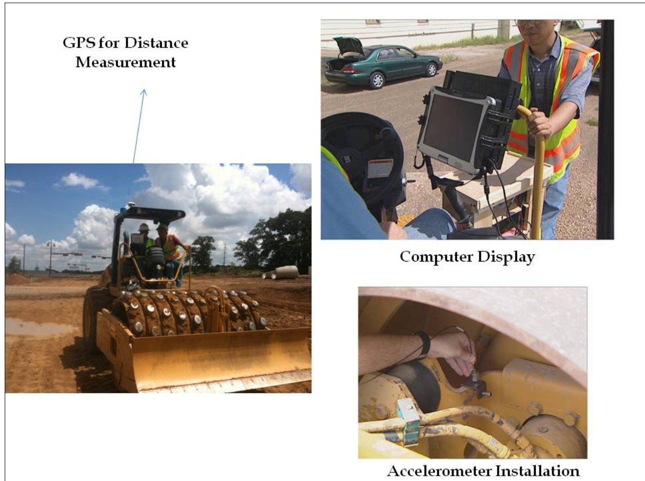
Figure 4. Components of the Instrumented Roller Package.
