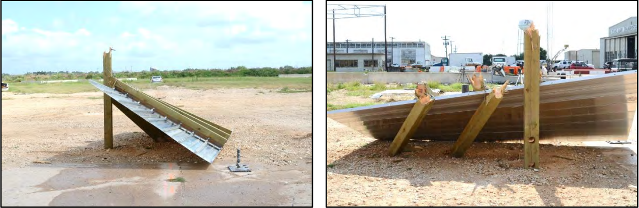
Figure 4.15. Modified Direct Embedded Wood Support Temporary Guide Sign System after Test No. 467823-2b.
