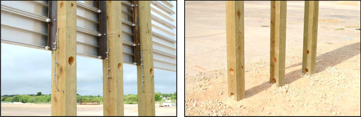
Figure 4.13. Modified Direct Embedded Wood Support Temporary Guide Sign System before Test Nos. 467823-2b and 467823-3.
