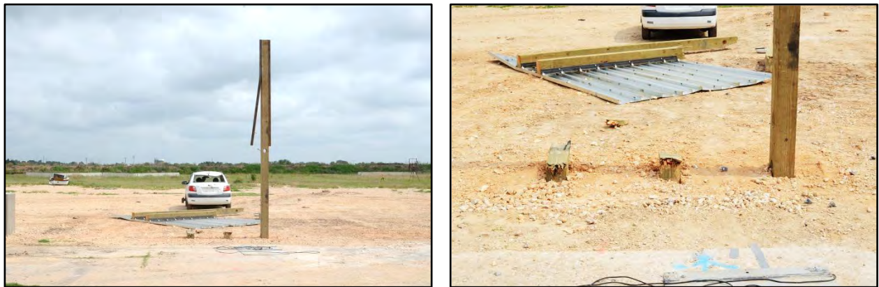
Figure 4.4. Direct Embedded Wood Support Temporary Guide Sign System after Test No. 467823-1.
