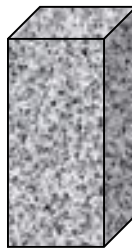
Figure 2-4. Example of a 5-Inches Long by 2-Inches Thick by 2-Inches Wide Prismatic Sample.
