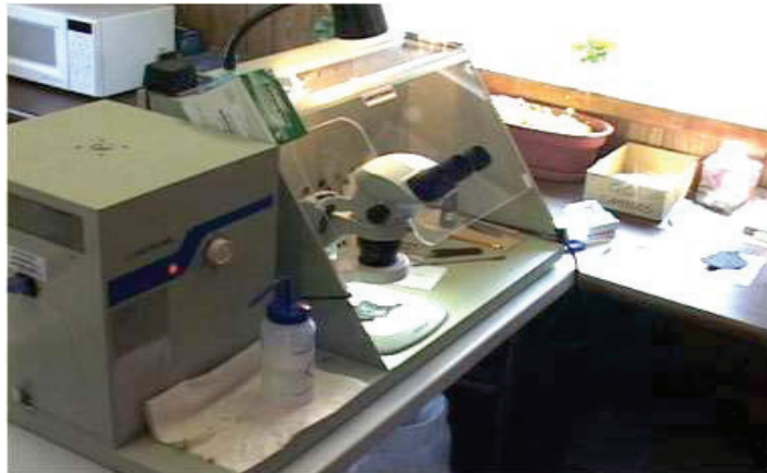
Figure 23. Setup for Asbestos Testing (13).
