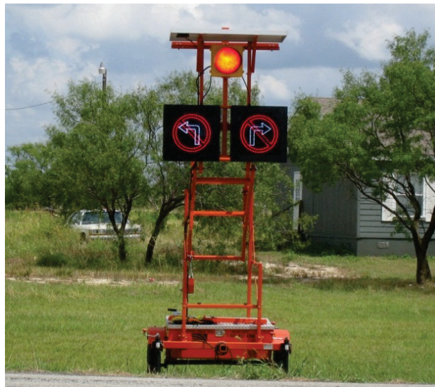
Figure 10. Blank-Out Sign Device in the Stop Phase.
