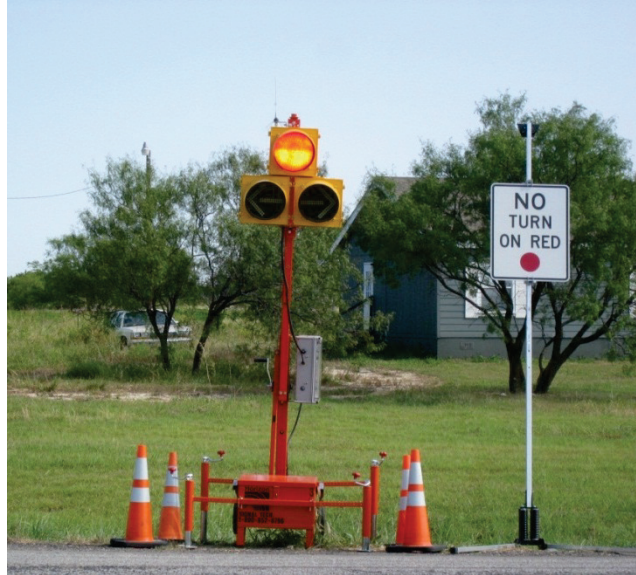
Figure 7. Modified Hybrid Device in the Stop Phase.
