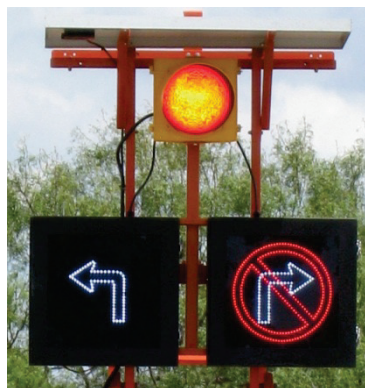
Figure 11. Blank-Out Sign Device Allowing a Left Turn.
