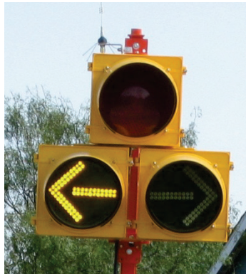
Figure 8. Modified Hybrid Device Allowing Left Turns.
