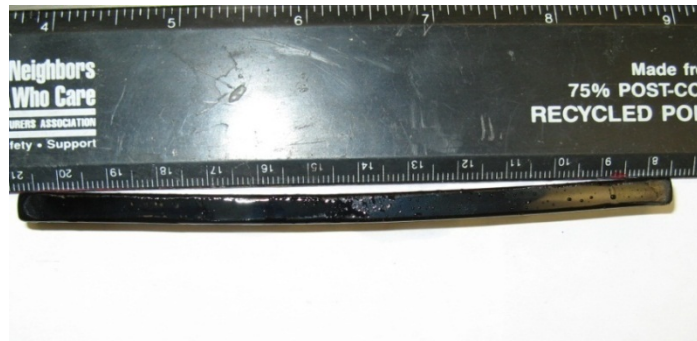
Figure A5. BBR Test: Early Fractured RAS Binder Beam.
