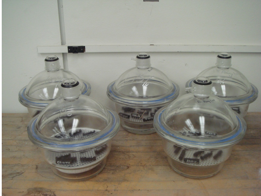
Figure 103. Moisture-Conditioned DMA Specimens in Desiccators.
