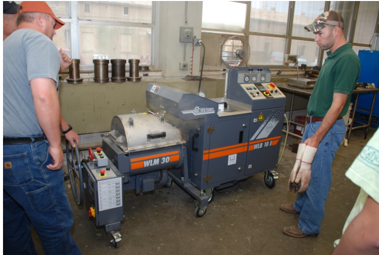
Figure 1. Wirtgen Laboratory Scale Foamed Bitumen Equipment in TTI's Laboratory.
