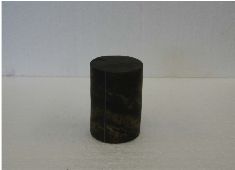
(b) Limestone Specimen Soaked in AAD Asphalt Binder for 32 Hours
