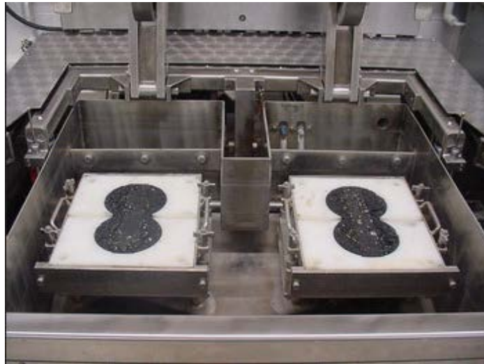
Figure 27. HWTT Machine with Cylindrical SGC Specimens.
