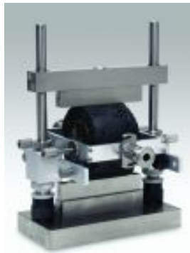
Figure 24. Schmidt Device for Measuring Resilient Modulus (ASTM D 4123).
